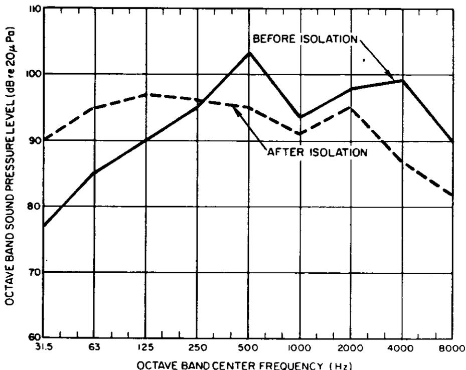
Figure 6.3.3. Quasi-peak levels 4 ft from press foot, before and after isolation.
