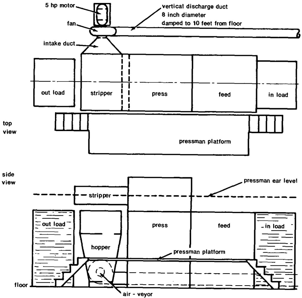
Figure 6.5.1. Scrap handling system for cutting press.
