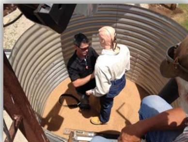
Kevin Moore applying pressure mapping measurement devices to dummy.
