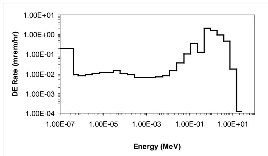
Figure 6-3. Neutron energy spectrum measured by PNL for drums of <sup>241</sup>Am-oxide in Building 3100 [7].
