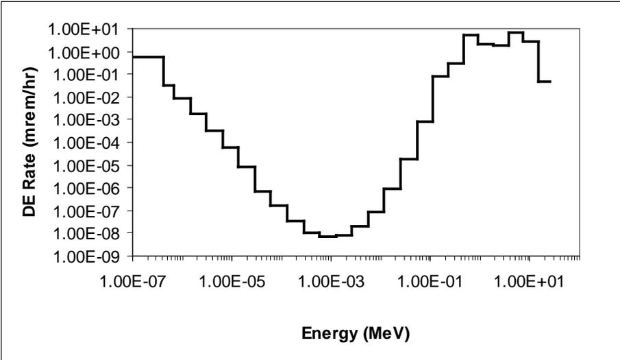
Figure 6-2. Neutron spectrum measured by PNL for <sup>238</sup>Pu:Be and <sup>252</sup>Cf sources in a water-shielded drum in Building 3038 [5].
