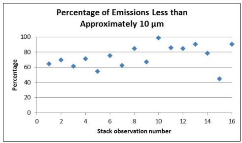
Figure 4-3. Percentage of stack emission less than approximately 10 µm AMAD (Spenceley 1985).
