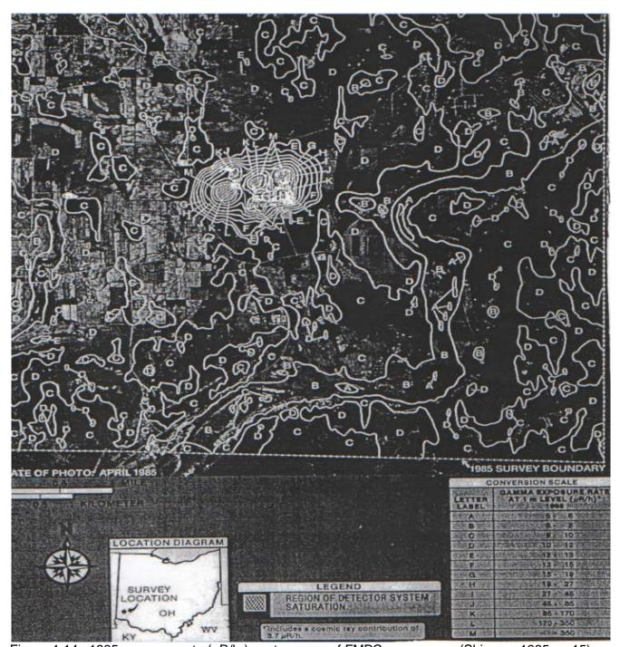
Figure 4-14. 1985 exposure rate (µR/hr) contour map of FMPC survey area (Shipman 1985, p. 15).
