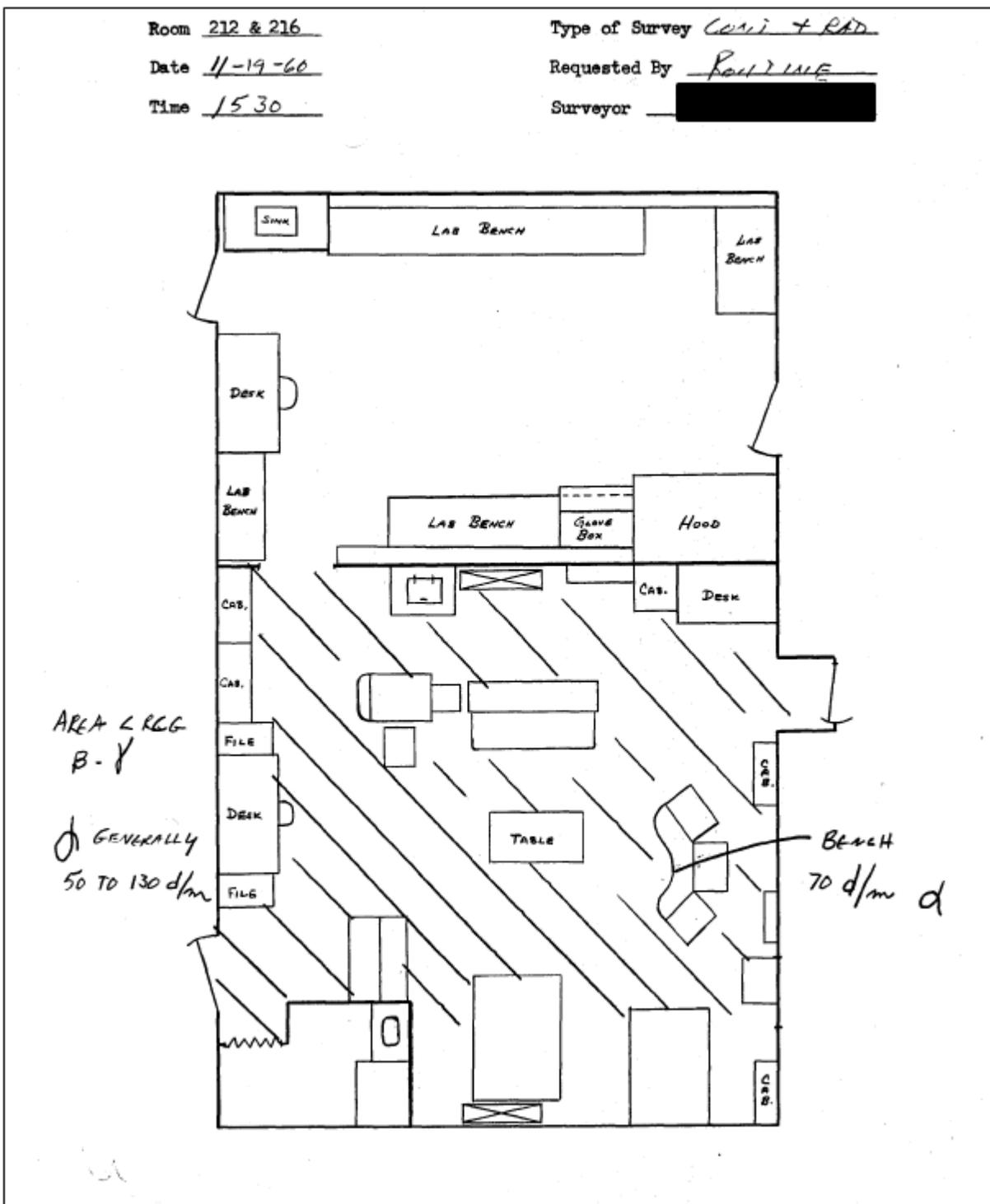
Figure 18: CPP-602 Room 212 and 216 Contamination Survey, November 19, 1960 (CPP 1960, page 6)
