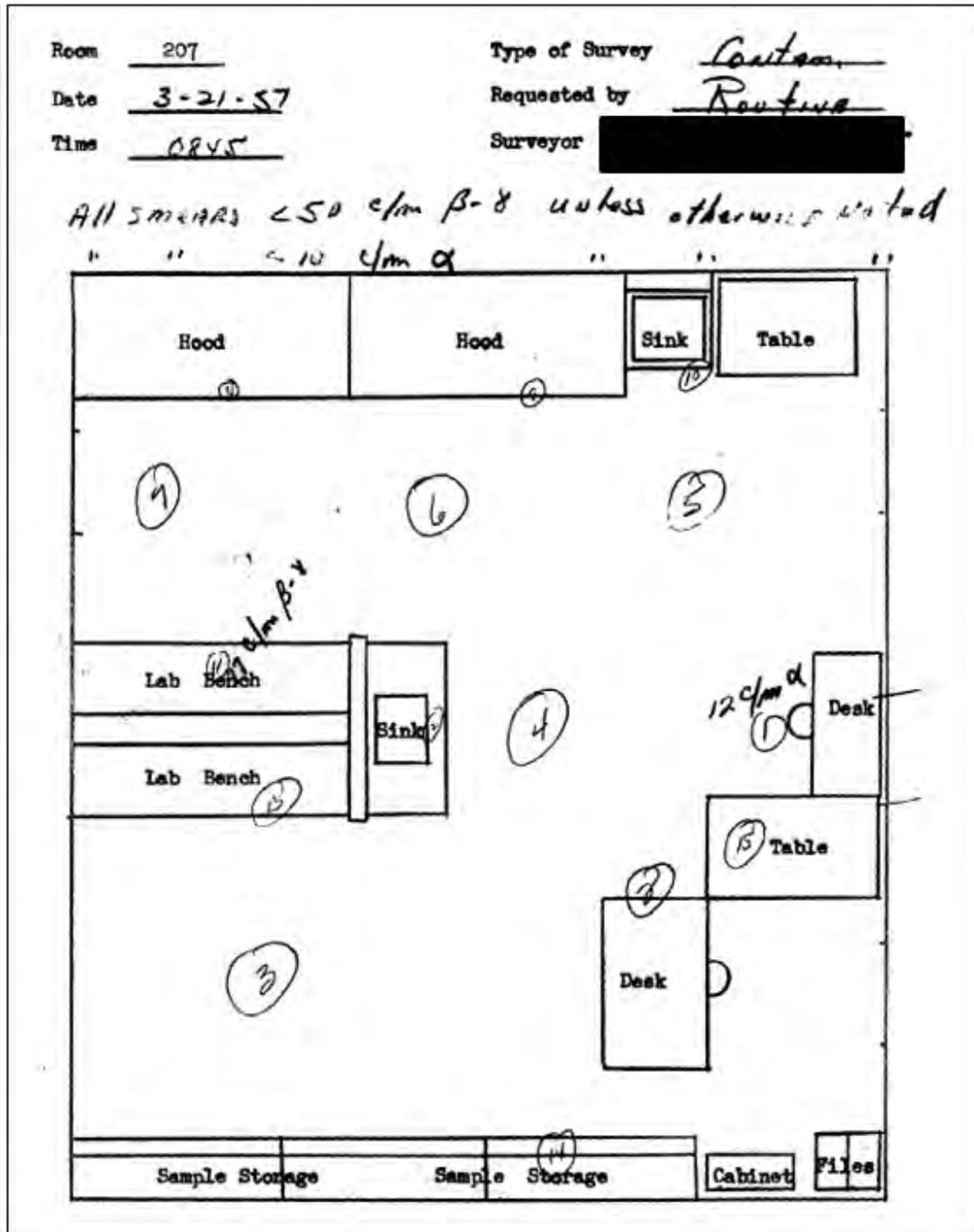
Figure 1: Contamination Survey of CPP Lab 207 in March 1957. (CPP 1957, page 6)
