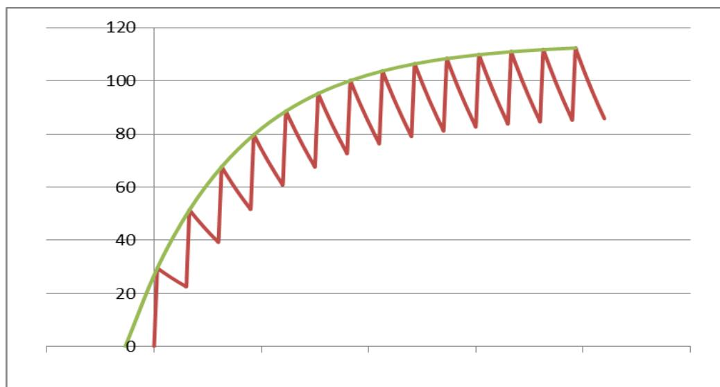
This new curve eventually reaches an equilibrium value of  $P_{eff}/$ . The effect of this adjusted production rate will depend on the half-life of the particular isotope. Table A1 below shows the adjustment for both the short and long shot scenarios for the longest and shortest lived isotopes
