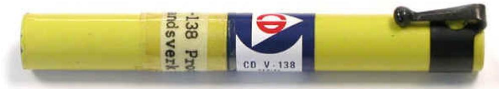
Figure 5 shows a drawing of a typical pocket dosimeter. The principle of the dosimeter is basically that of an electroscope. A charge is put on the fibers where one fixed and one movable fiber repel each other. As ionizing radiation ionizes the air in the chamber, the charge is collected on the fibers and they repel each other a little less. As the charge is lessened, the movable fiber casts a shadow across a scale showing a higher dose.
