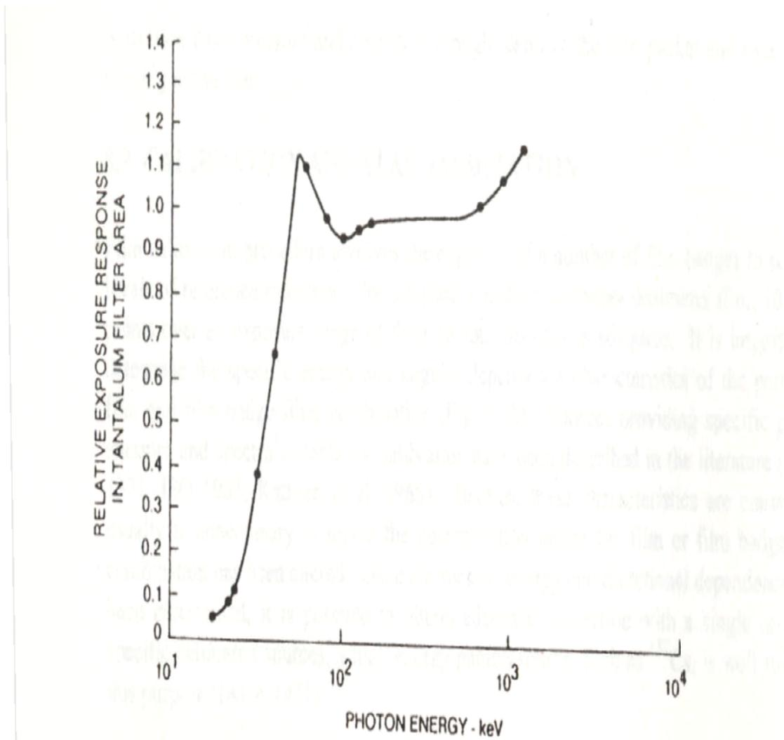
Film response with 0.020 inch tantalum filter (adapted from Brady and Iverson 1968)
