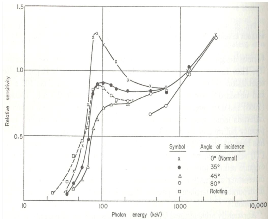
Relative sensitivity of Kodak RM film as a function of photon energy and angle of incidence of radiation. Film under filter of 0.71 mm Sn plus 0.31 mm Pb. (Heard and Jones, 1963)<sup>2</sup>
