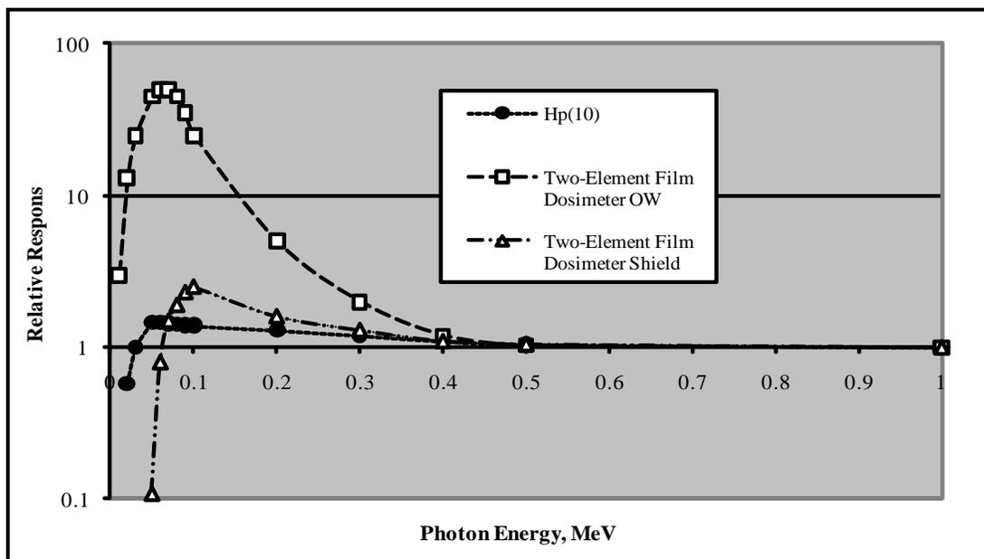
Figure 2-1. Measured two-element dosimeter photon response for anterior-to-posterior exposure geometry (Pardue et al 1944, Wilson et al 1990).
