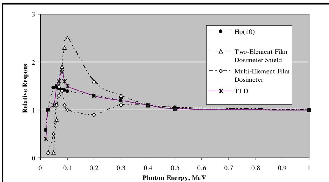
Figure 2-2. Measured deep dose response for Hanford Two-Element film, multi-element film and thermoluminescent dosimeter compared to  $H_p(10)$ . (Wilson et al 1990).
