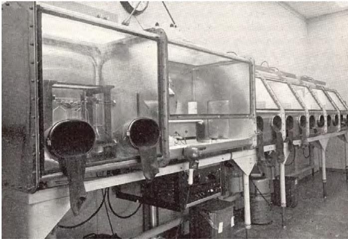
Figure 4 Plutonium gloveboxes at LANL's CMR facility<sup>(1)</sup>
