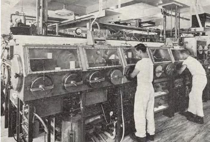
Figure 1 Plutonium gloveboxes at LANL <sup>(1)</sup>
