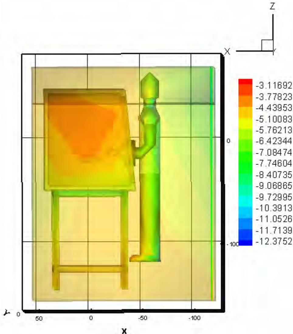
Figure 7 ATTILA model geometry and flux contours
