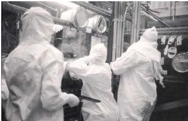
Figure 3 Plutonium gloveboxes at Hanford <sup>(2)</sup>
