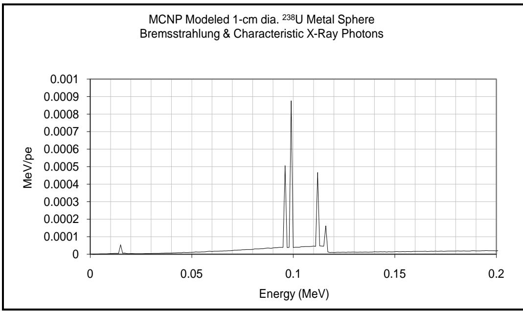
Figure 6-8. Characteristic X-ray component of calculated spectrum from  $^{238}\text{U}$  spheres on linear vertical axis. Source: Calculations made using Los Alamos 2003.
