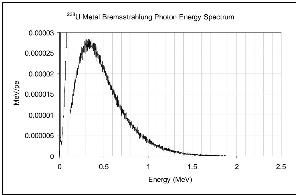
Figure 6-7. *Bremsstrahlung* component of calculated spectrum from  $^{238}\text{U}$  spheres on linear vertical axis. Source: Calculations made using Los Alamos 2003.
