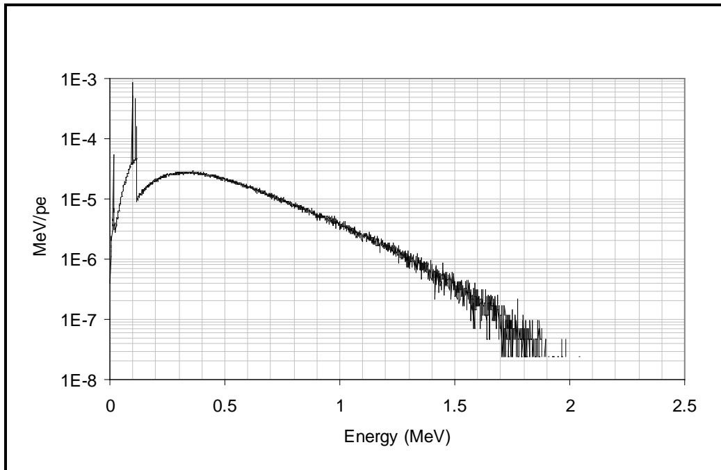
Figure 6-6. MCNP-calculated photon spectra emitted from  $^{238}\text{U}$  as excited by  $^{234\text{m}}\text{Pa}$  beta in  $^{238}\text{U}$  spheres. Source: Calculations made using Los Alamos 2003.
