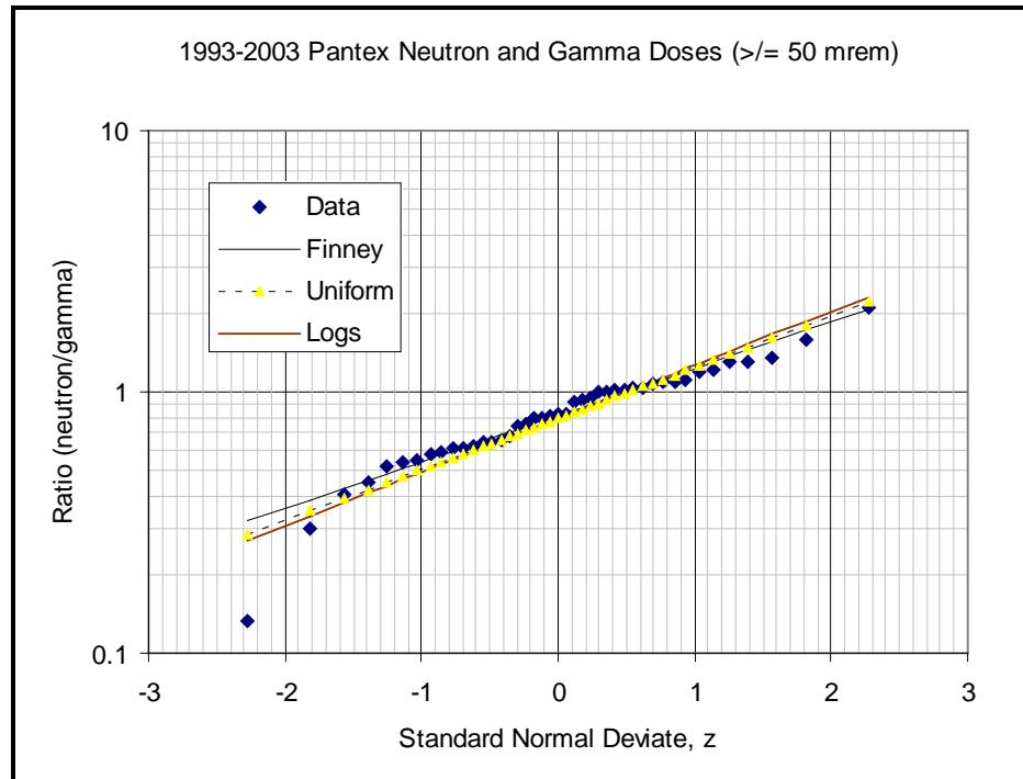
Figure 6-10. Log-probability plot of grouped neutron-to-photon dose ratios. Source: Strom 2004.
