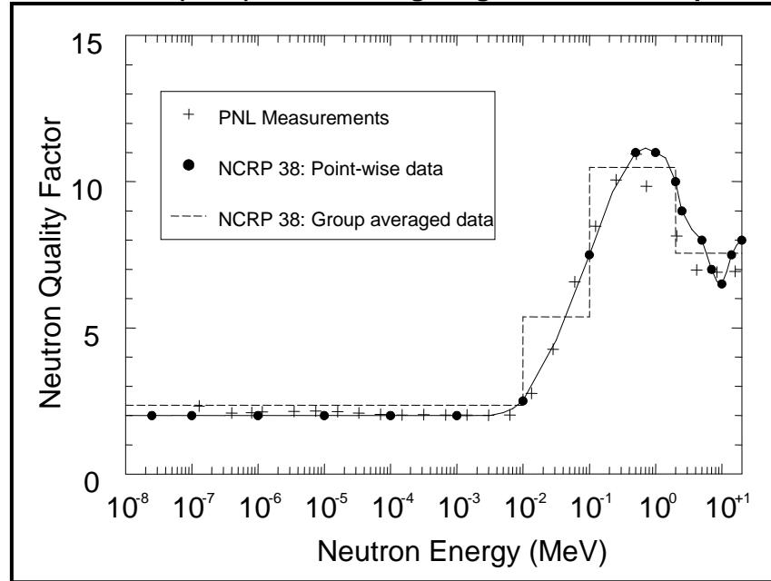
Figure 6-11. Comparison of neutron quality factors used in PNL neutron spectrum measurements (Soldat et al 1990) and neutron quality factors from NCRP (1971), shown as point-wise data and grouped averaged data over four neutron energy groups used in dose reconstruction for Y-12 Plant workers.
