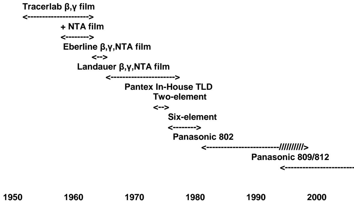
Figure 2-6. Evolution of external dosimetry at Pantex
