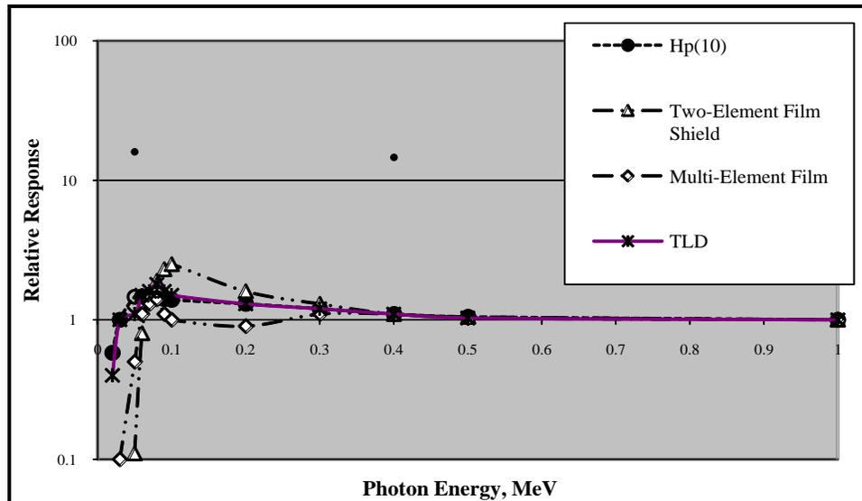
Figure 6-1. Estimated dosimeter photon response characteristics.
