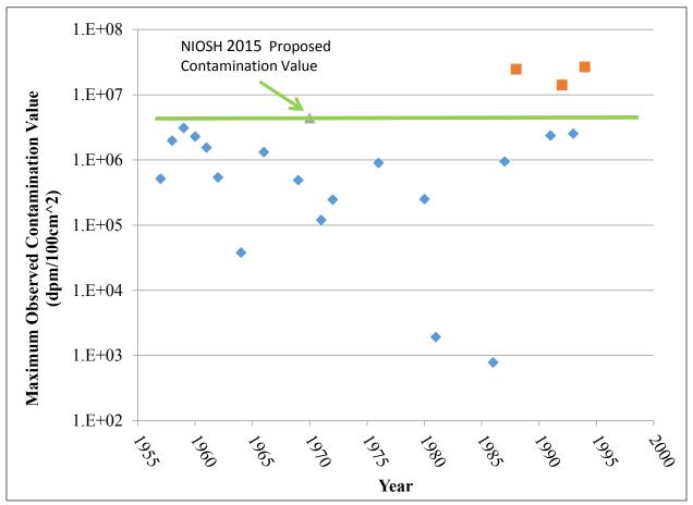
Figure 4. Maximum Observed Contamination Value by Year in dpm/100cm<sup>2</sup>
