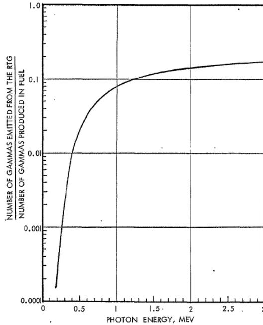
Figure 4-8. Ratio of Number of Gamma Escaping the RTG to Number of Gammas Produced in the Fuel for a Pair of SNAP-19 RTG's at 20° to the Longitudinal Axis.
