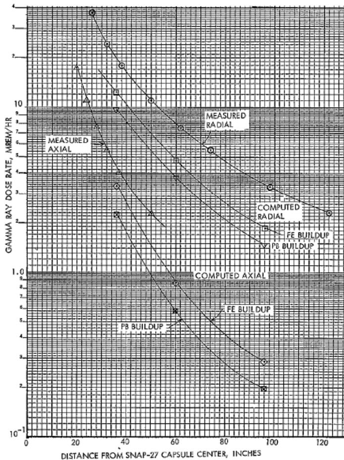
Figure 4-10. Gamma Dose Rates vs. Distance From the Center of a SNAP-27 Capsule
