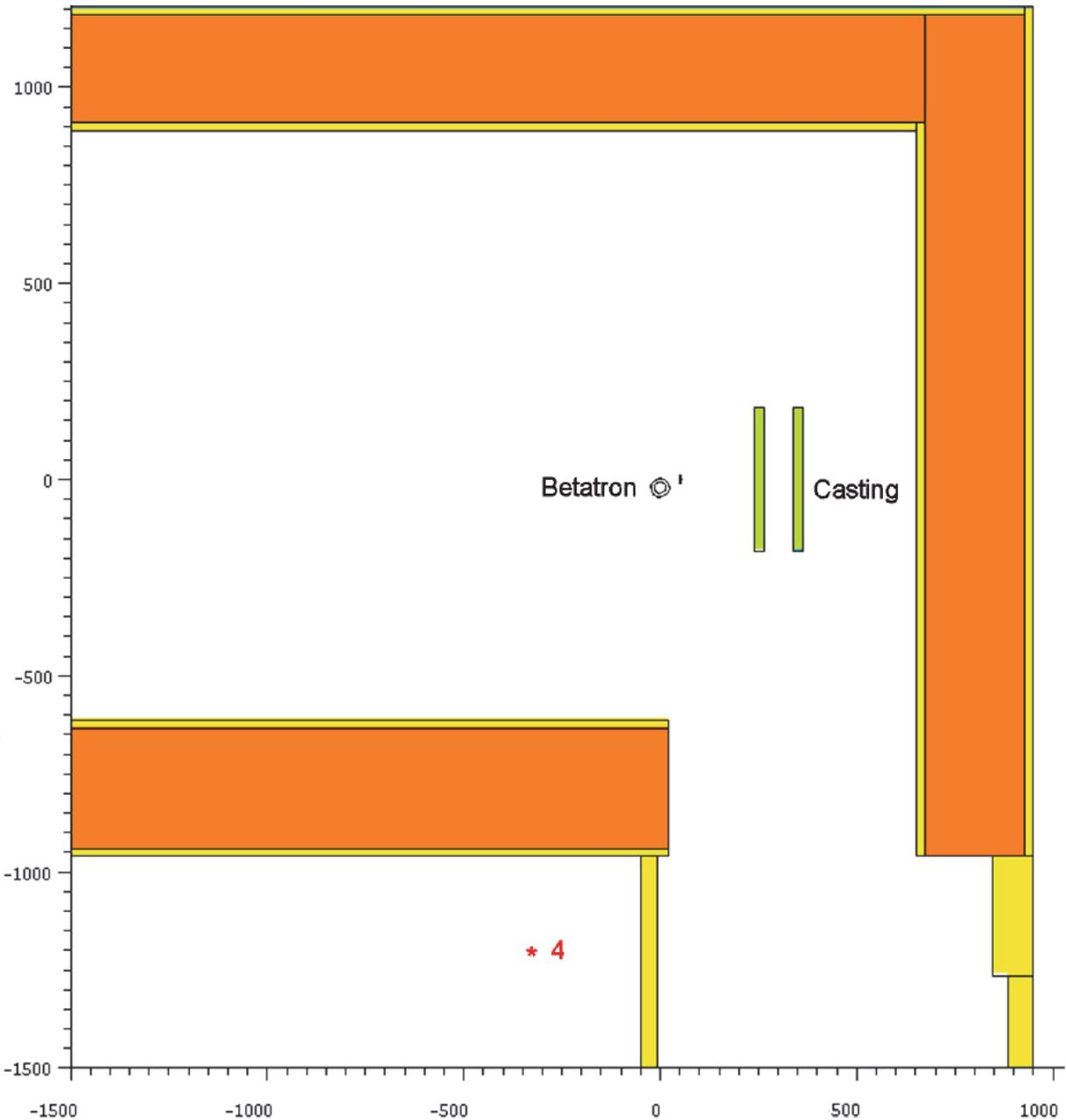
Figure 4. MCNPX Model of Radiography of Steel Casting in New Betatron Building (scales in cm)
