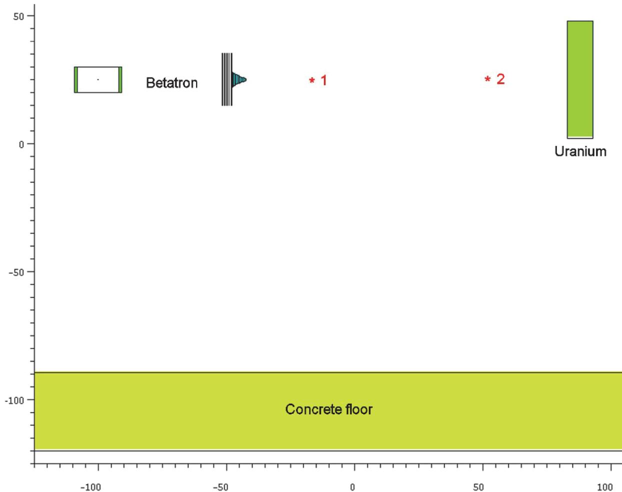
Figure 1. MCNPX Model of Exposure to Irradiated Uranium in Old Betatron Building (scales in cm)
