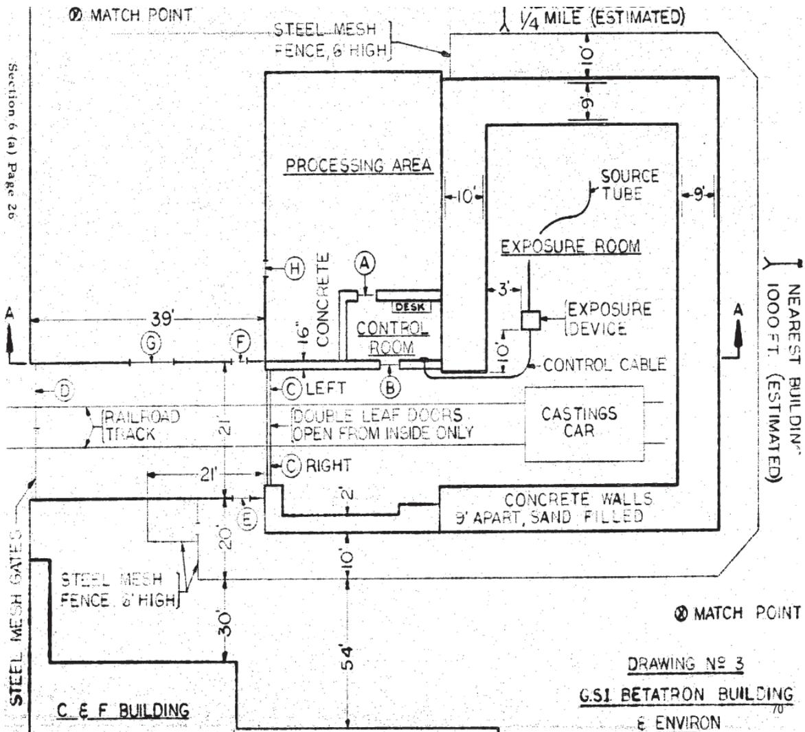
Figure 3. Drawing of New Betatron Building Showing Desk in Control Room (NRC 2009)
