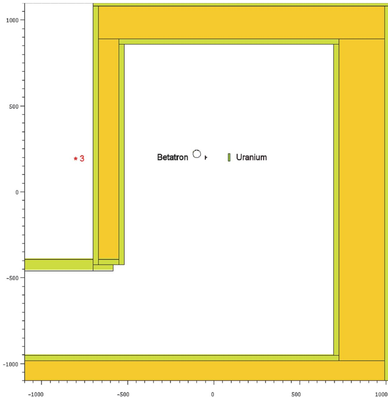
Figure 2. MCNPX Model of Radiography of Uranium in Old Betatron Building (scales in cm)
