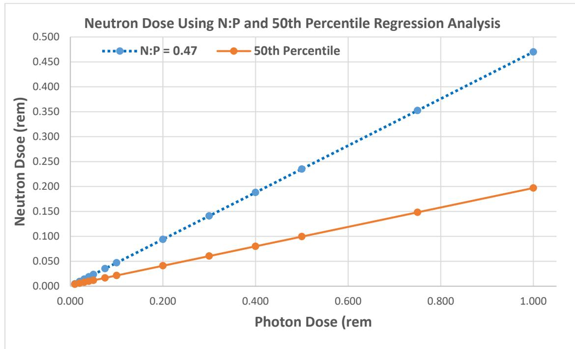
As can be seen from this example, the use of the QRA method results in approximately half the neutron dose being assigned compared to using the standard N:P ratio method.
