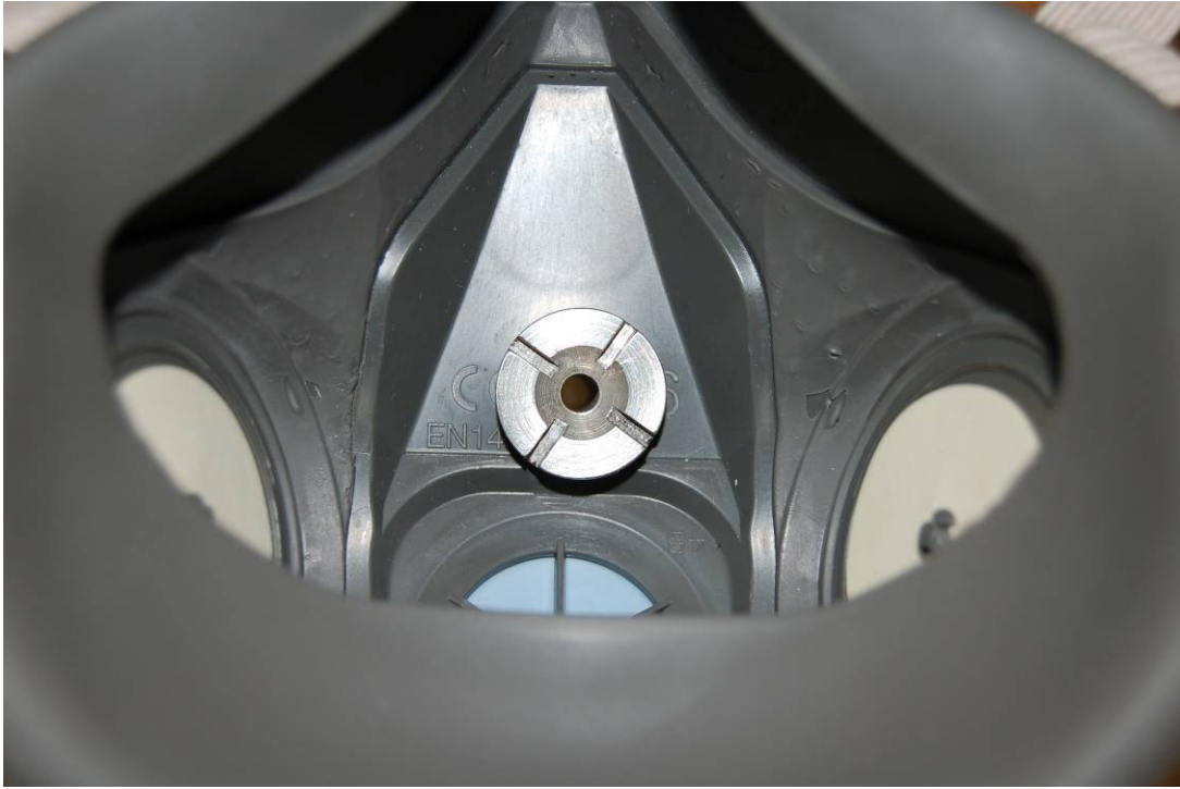
Figure 7: Interior View of a Sample Respirator Probed
