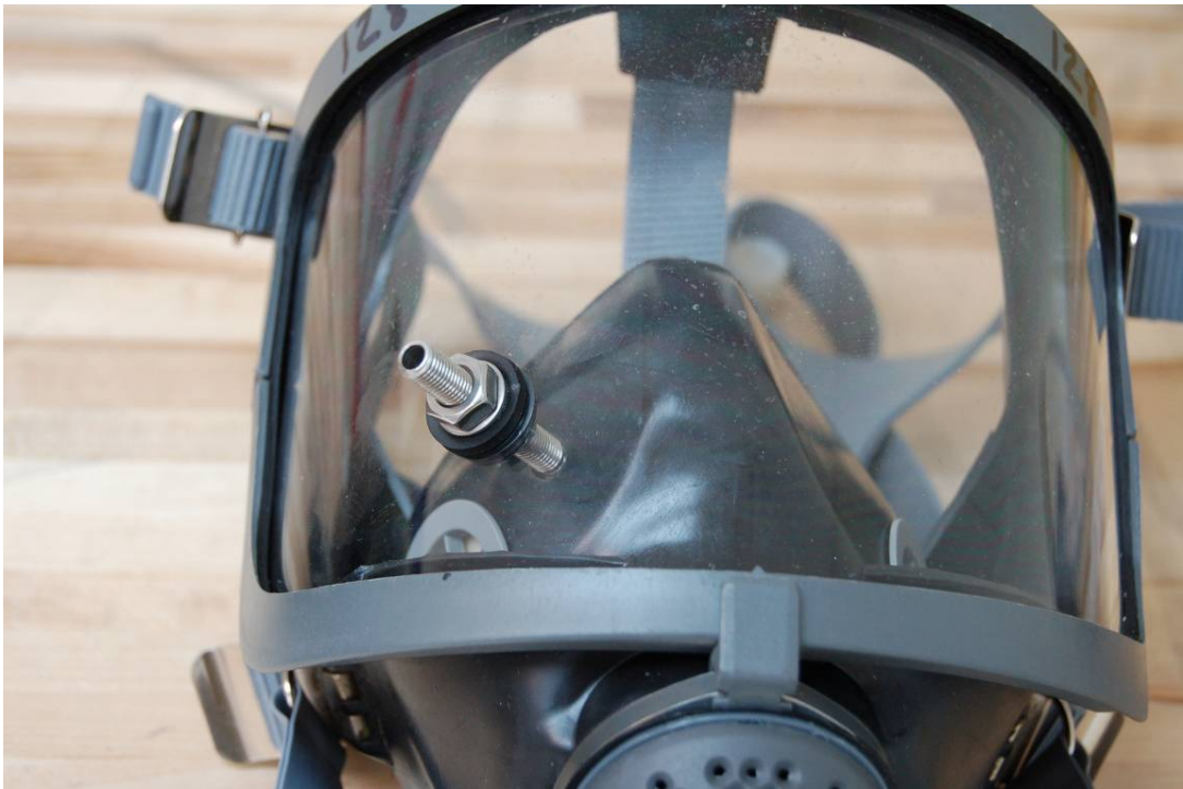
Figure 7: Interior View of a Sample Respirator Probed
