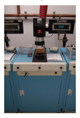
8.3. Photograph - Close up of respirator test fixture in the closed chuck
