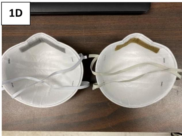
**Fig. 1D. Nose Foam Discoloration (Left-Control, Right-Treated)**
