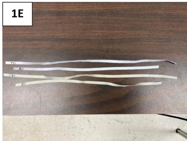
**Fig. 1E. Strap Discoloration (Top-Control, Bottom-Treated)**
