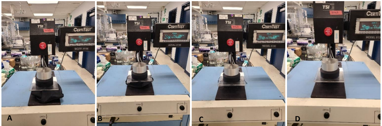
Figure 2: Laboratory Test Photo (TSI, Inc. 8130 filter tester). A) Bal-Blk-A, Balaclava-style Mask. B) Bnd-Blk-A, Bandana-style Mask. C) Loop-Blk, Ear Loop-style Mask. D) Filter only as provided for testing.
