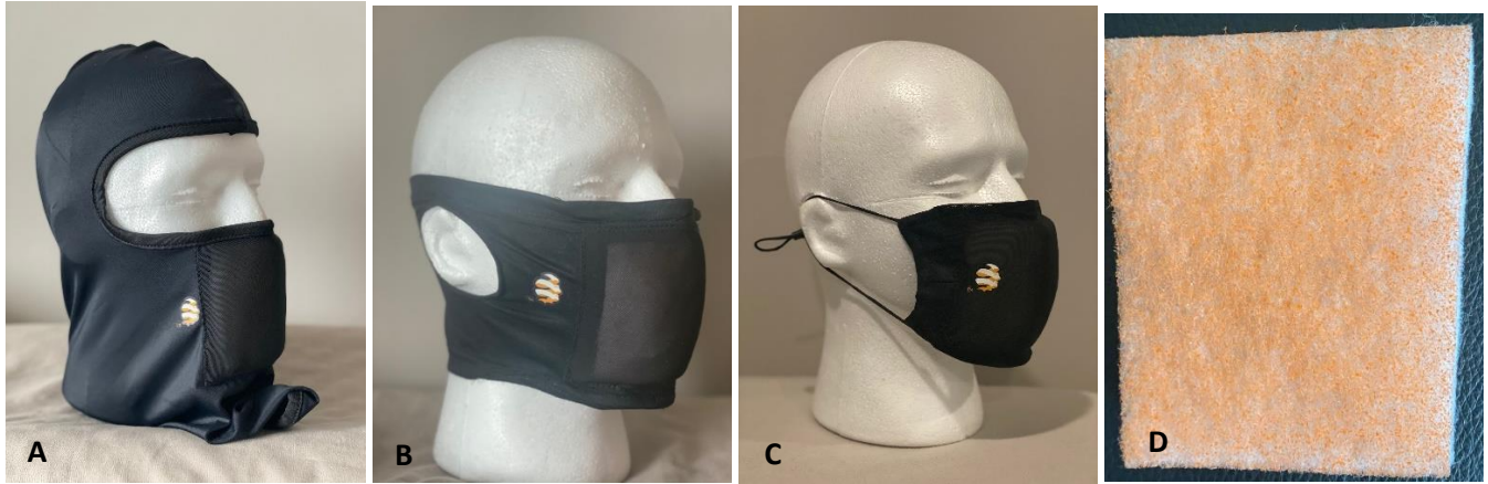
Figure 1: Masks evaluated. A) Bal-Blk-A, Balaclava-style Mask. B) Bnd-Blk-A, Bandana-style Mask. C) Loop-Blk, Ear Loop-style Mask. D) Filter only as provided for testing.
