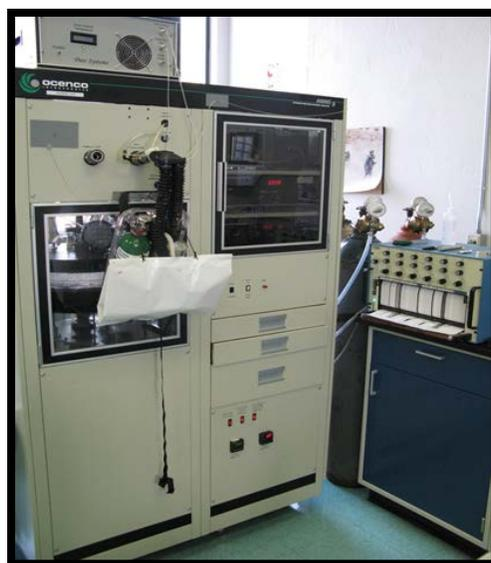
Figure 5. Automated Breathing and Metabolic Simulator
