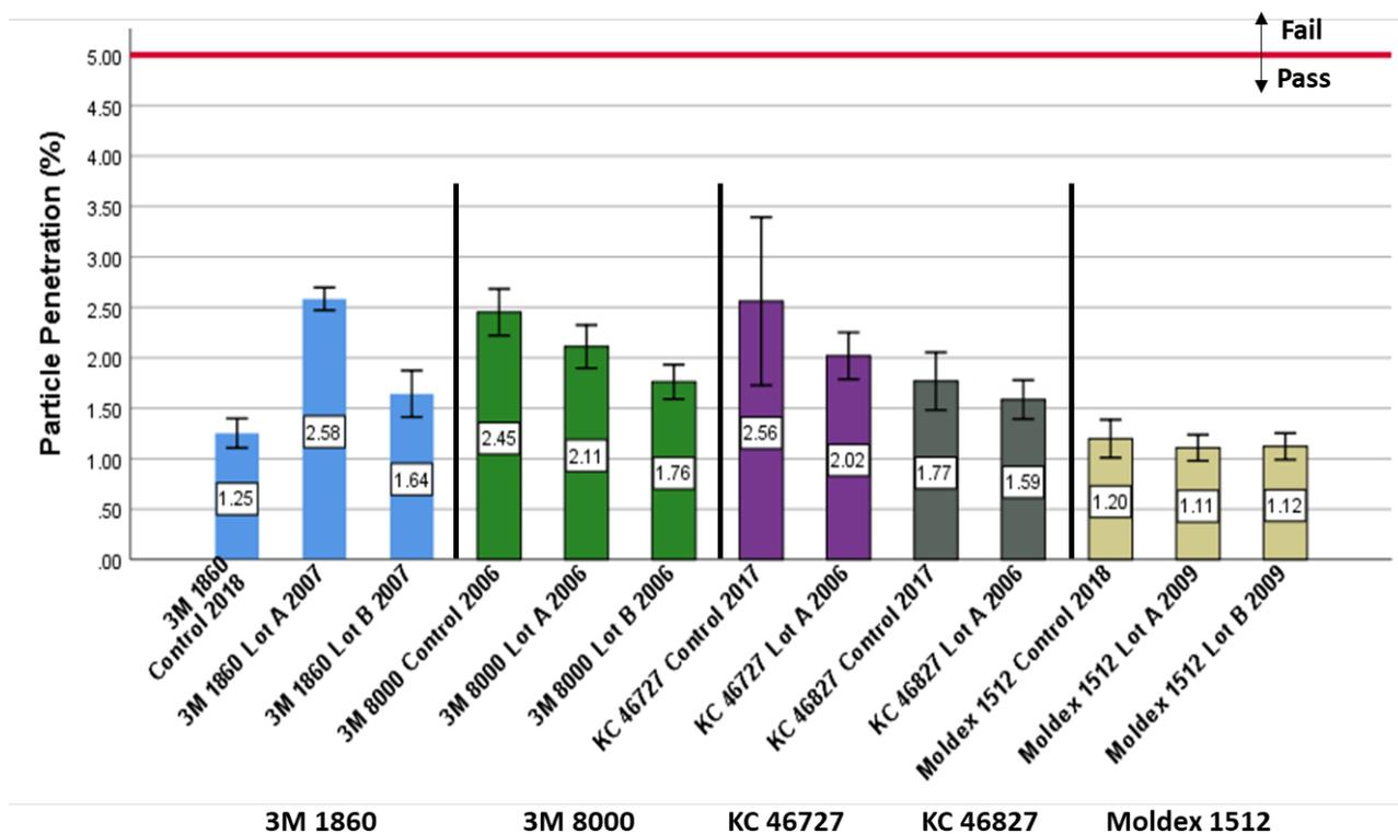
**Figure 7:** Control and stockpiled respirator particle filtration performance data. N95 FFRs must have a particle penetration of less than 5.0%. Error bars represent the 99% confidence interval and estimate the population parameters. This confidence interval suggests that 99% of any repeated samples tested and evaluated from this lot will have a mean between the upper and lower bounds.
