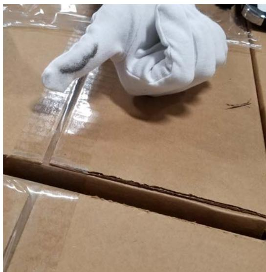
**Figure 2:** Most amount of dust observed on product cases from Facility Six.
