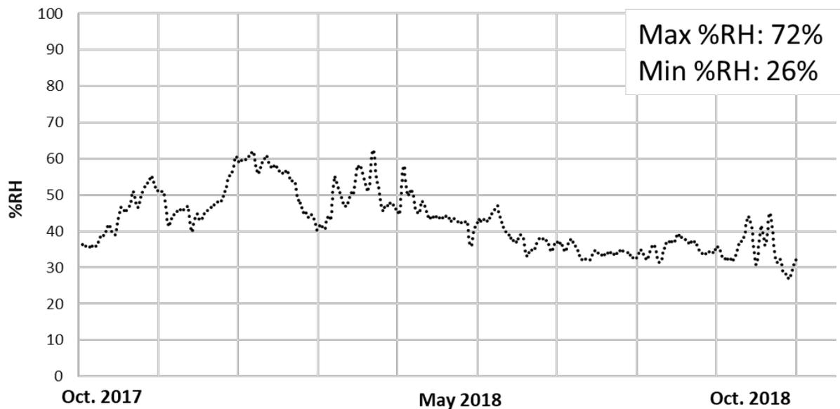
**Figure 4:** Percent Relative Humidity (% RH) from October 2017 – October 2018 for two data loggers stored at Facility Five. Data is plotted as a 50-point moving average for visualization purposes. Maximum and minimum temperatures reported are noted for each data logger.
