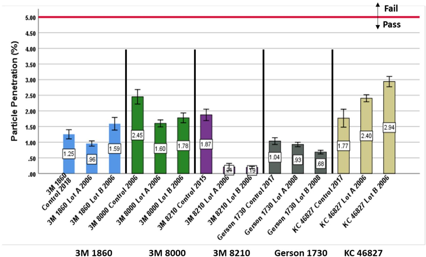
**Figure 6:** Control and stockpiled respirator particle filtration performance data. N95 FFRs must have a particle penetration of less than 5.0%. Error bars represent the 99% confidence interval and estimate the population parameters. This confidence interval suggests that 99% of any repeated samples tested and evaluated from this lot will have a mean between the upper and lower bounds.
