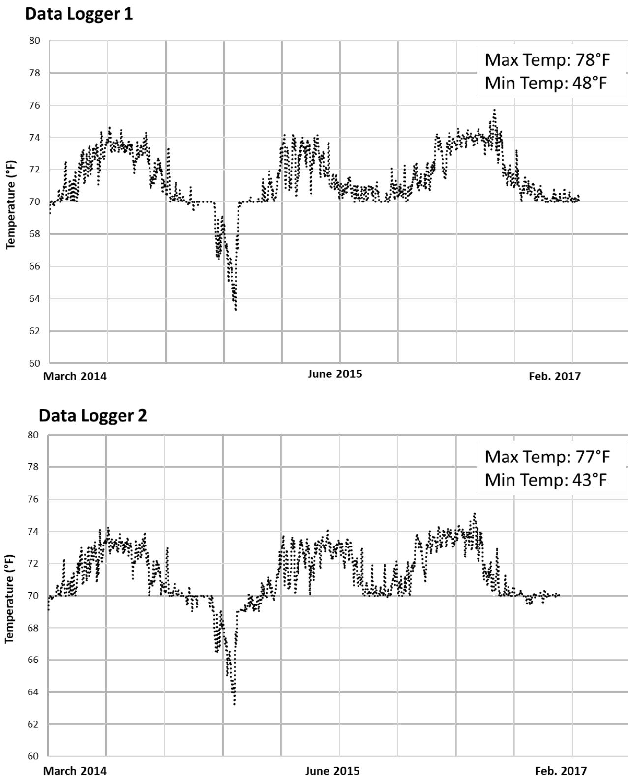
**Figure 6:** Temperatures from March 2014 – February 2017 for two data loggers stored at Facility One. Data is plotted as a 50-point moving average for visualization purposes. Maximum and minimum temperatures reported are noted for each data logger.
