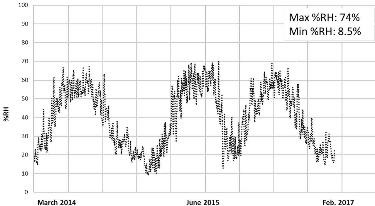
**Figure 5:** Percent Relative Humidity (% RH) from March 2014 – February 2017 for two data loggers stored at Facility One. Data is plotted as a 50-point moving average for visualization purposes. Maximum and minimum temperatures reported are noted for each data logger.
