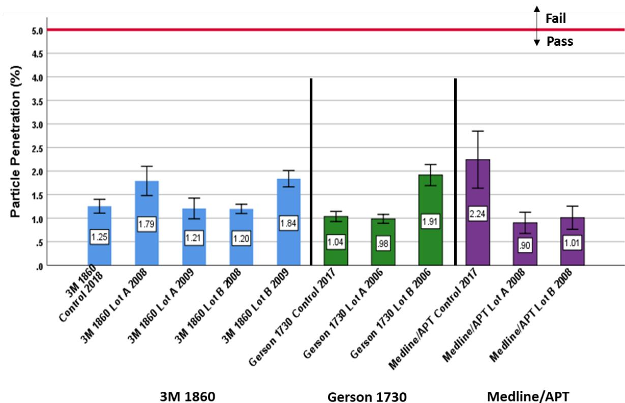
**Figure 8:** Control and stockpiled respirator particle filtration performance data. N95 FFRs must have a particle penetration of less than 5.0%. Error bars represent the 99% confidence interval and estimate the population parameters. This confidence interval suggests that 99% of any repeated samples tested and evaluated from this lot will have a mean between the upper and lower bounds.
