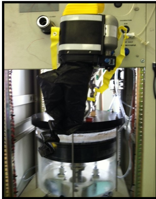
Figure 4. Front view of Ocenco M-20.2 breathing bag stuck in folded position
