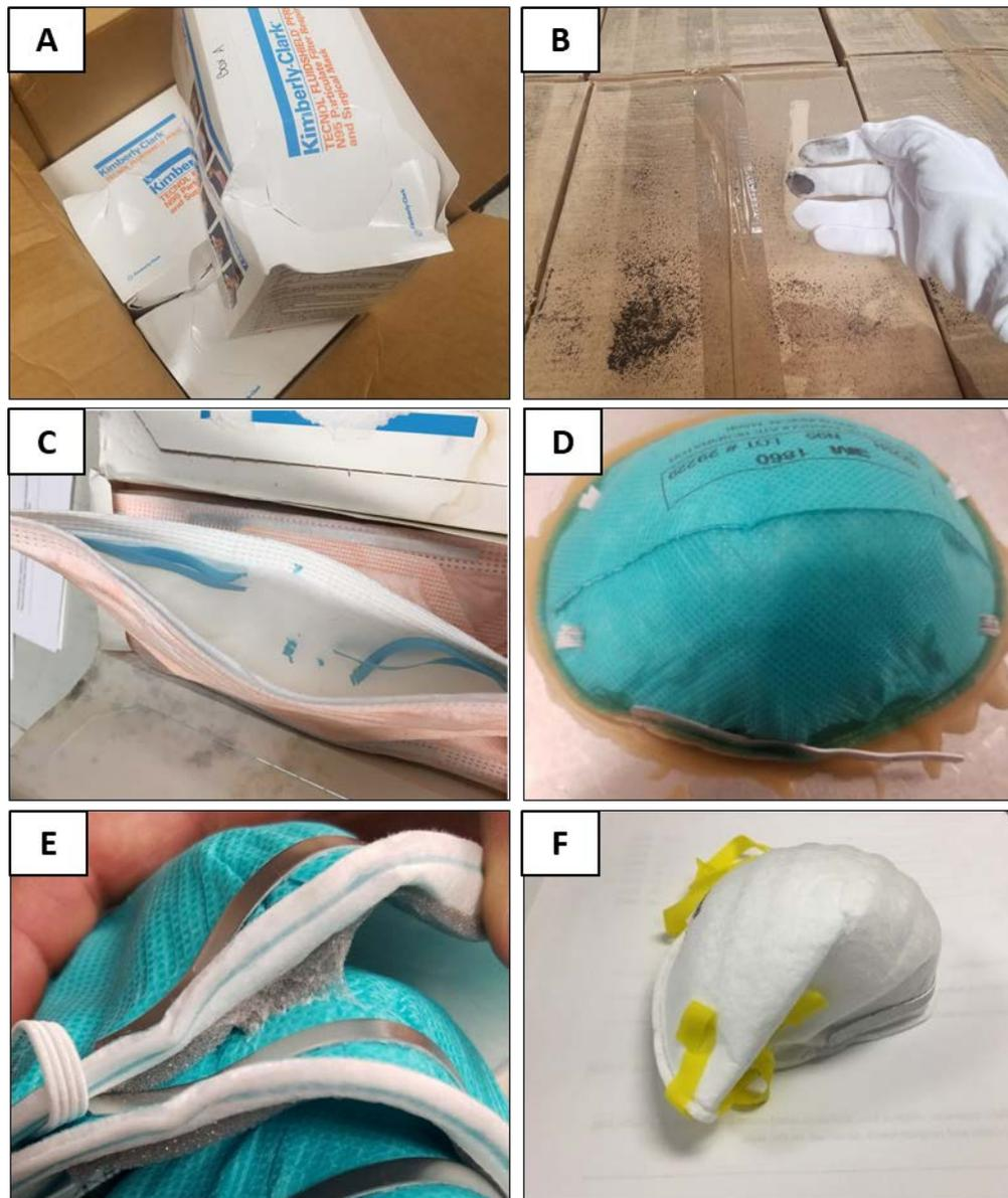
**Figure 3:** Examples of visual inspection concerns to the respirator box and individual respirator units including A) box damage; B) dust; C) strap damage to respirator and mold on respirator box; D) damage to respirator nose bridge (here, the respirator is fixed to test plate); E) damage to respirator nose foam; and F) crushing of the respirator unit itself.
