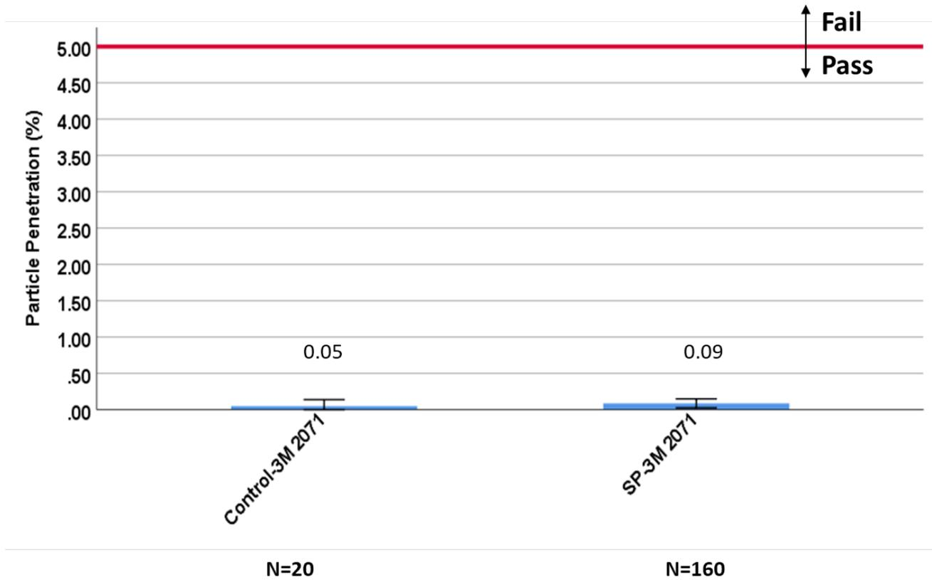
**Figure 9:** Mean control and stockpiled (SP) respirator particle filtration performance data for the 3M 2071 model. P95 filters must have a particle penetration of less than 5.0%. Error bars represent the 99% confidence interval and estimate the population parameters. This confidence interval suggests that 99% of any repeated samples tested and evaluated from this lot will have a mean between the upper and lower bounds. The number of units tested is shown under the model name.
