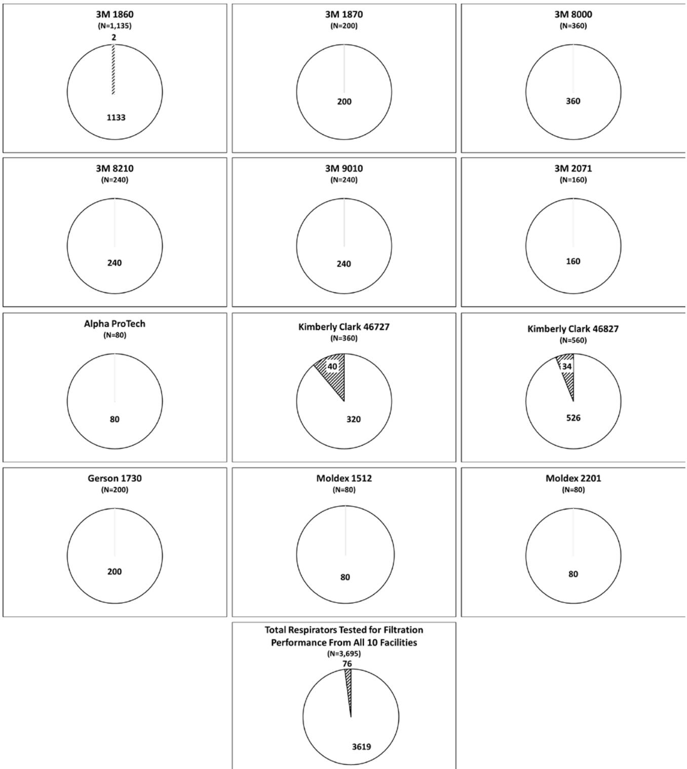
**Figure 11:** Summary of the stockpiled respirators tested for **filtration efficiency performance** from twelve APR models, as well as the total stockpiled respirators tested for **filtration efficiency performance** across the ten facilities. White represents the number of passing respirators and the black lines represents the number of failing respirators for each model.
