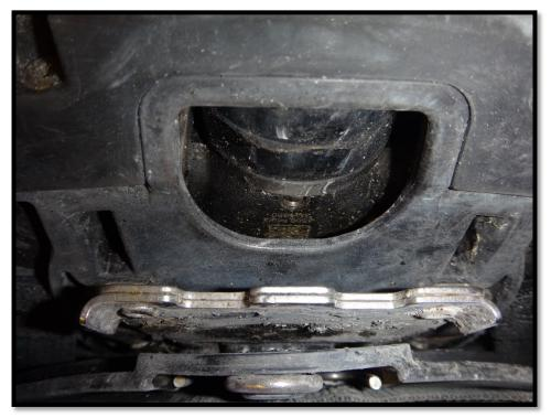
Figure 11: Bottom view of pressure reducer assembly
