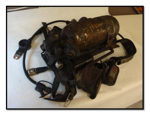
Figure 29: Overview of straps and cylinder connected to SCBA
