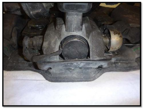
Figure 10: Pressure reducer, RIC UAC with primary low pressure warning device (bell)
