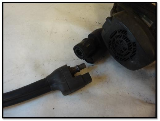
Figure 9: Low pressure line disconnected from intermediate pressure hose
