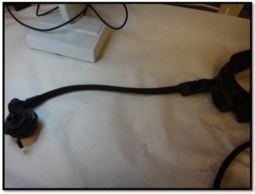
Figure 8: Mask mounted regulator and low pressure line connected to SCBA
