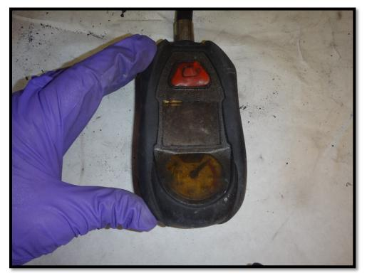
Figure 13: Front of PASS control module
