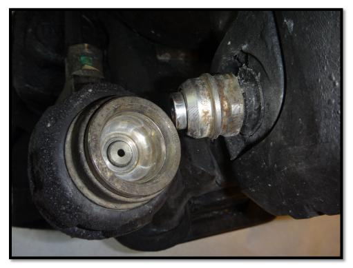
Figure 17: Cylinder attachment and Quick Connect adapter
