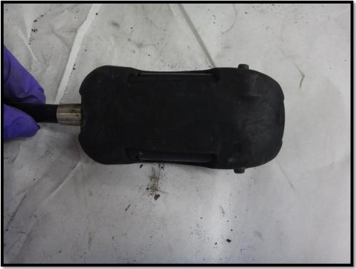
Figure 14: Back of PASS control module
