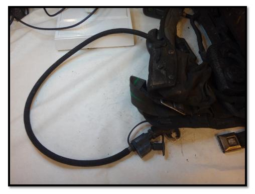
Figure 19: ExtendAire II EBSS hose with male and female Quick Connect
