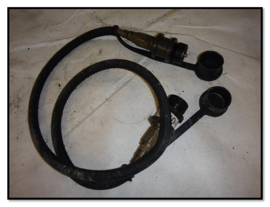
Figure 24: Quick-Fill hose with covers off
