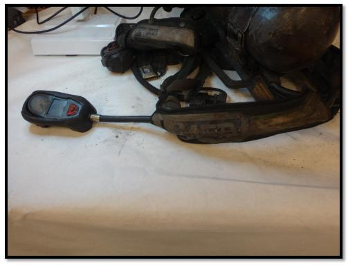
Figure 12: PASS control module and medium pressure line
