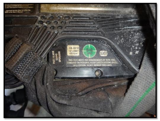
Figure 25: PASS power module SEI label
