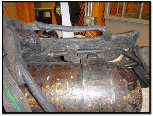
Figure 28: Cylinder strap and heat damage to side rail
