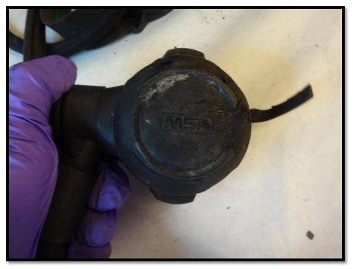
Figure 6: Mask mounted regulator with signs of heat damage
