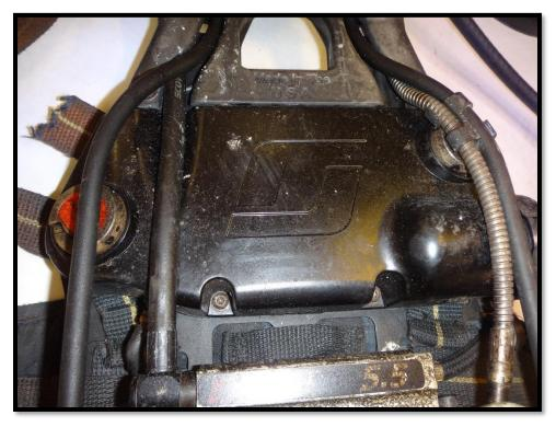
Figure 13: PASS control module.
