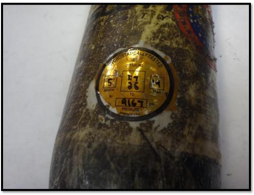
Figure 21: Cylinder hydrostatically tested label.
