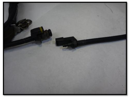
Figure 8: Low-pressure hose with quick disconnect (disconnected).
