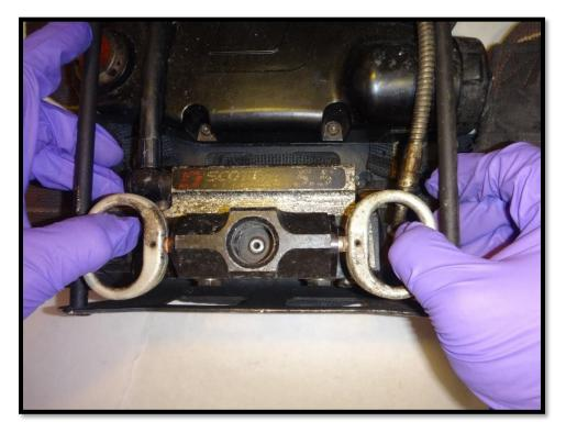
Figure 18: Cylinder snap-change connector.
