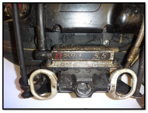
Figure 9: Pressure reducer.
