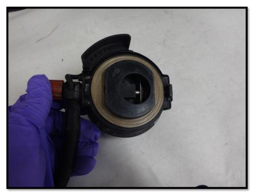
Figure 6: Inside seal of mask-mounted regulator and HUD.
