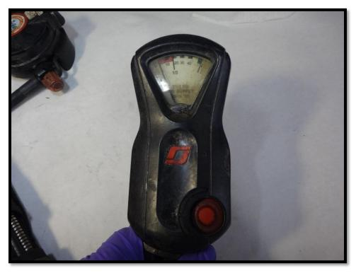
Figure 11: PASS control console.
