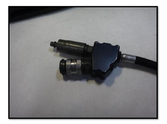
Figure 10: Dual Emergency Breathing Safety System (EBSS).
