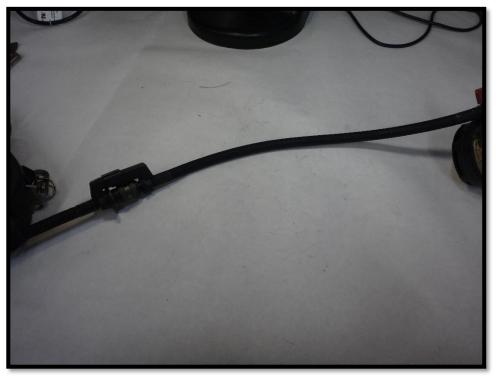
Figure 7: Low-pressure hose with quick disconnect (connected).
