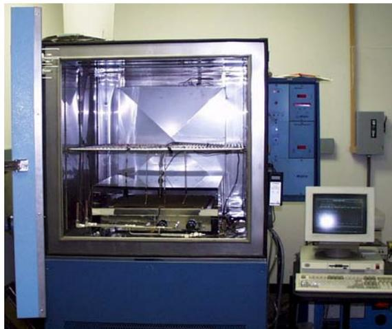
Figure 8. Guarded Sweating Hot Plate in Environmental Chamber
