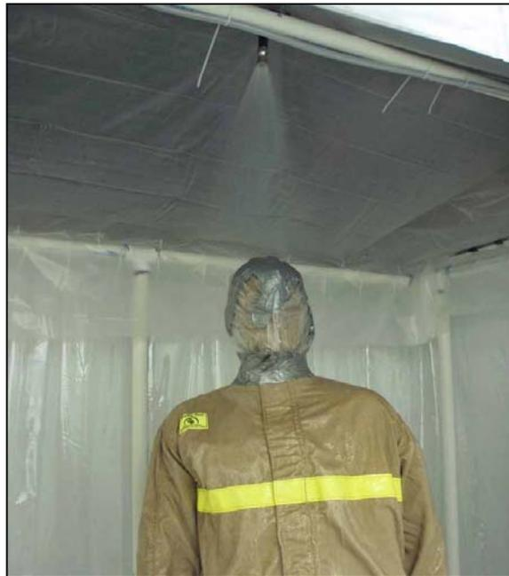
Figure 7. Liquid Integrity Test Used for Firefighter Protective Clothing
