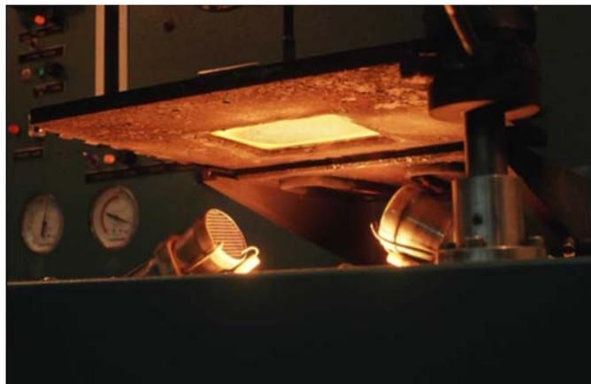
Figure 1. Thermal Protective Performance Tester.
