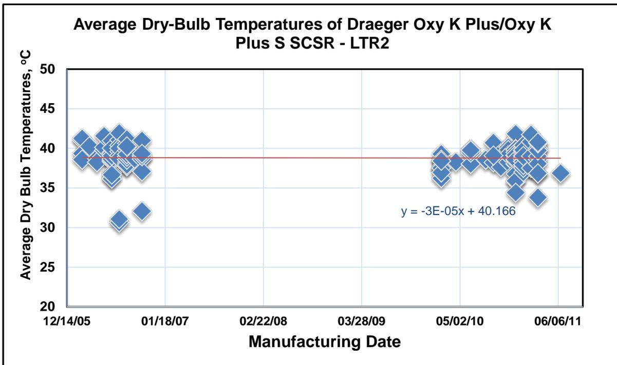
Figure 12. 60-Minute Average Dry-Bulb Temperatures of Field Deployed and New Dräger Oxy K Plus/Oxy K Plus S Self-Contained Self-Rescuers
