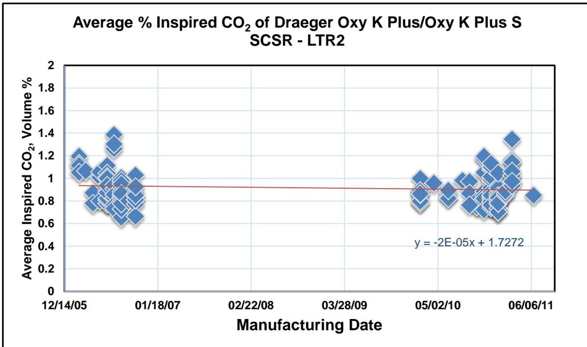
Figure 10. 60-Minute Average Percent Inspired Carbon Dioxide of Field Deployed and New Dräger Oxy K Plus/Oxy K Plus S Self-Contained Self-Rescuers
