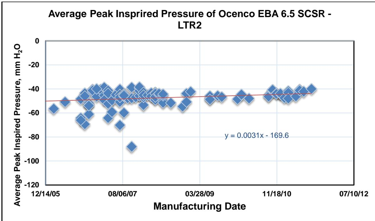
Figure 19. 60-Minute Average Peak Inspired Pressure of Field Deployed and New Ocenco EBA 6.5 Self-Contained Self-Rescuers
