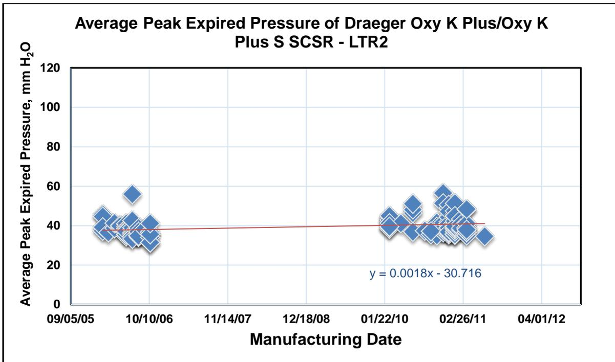
Figure 14. 60-Minute Average Peak Expired Pressure of Field Deployed and New Dräger Oxy K Plus/Oxy K Plus S Self-Contained Self-Rescuers
