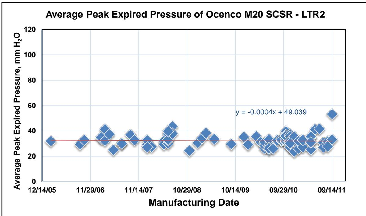
Figure 26. 10-Minute Average Peak Expired Pressure of Field Deployed and New Ocenco M-20 Self-Contained Self-Rescuers
