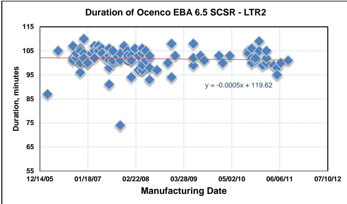
Figure 15. Duration of Field Deployed and New Ocenco EBA 6.5 Self-Contained Self-Rescuers
