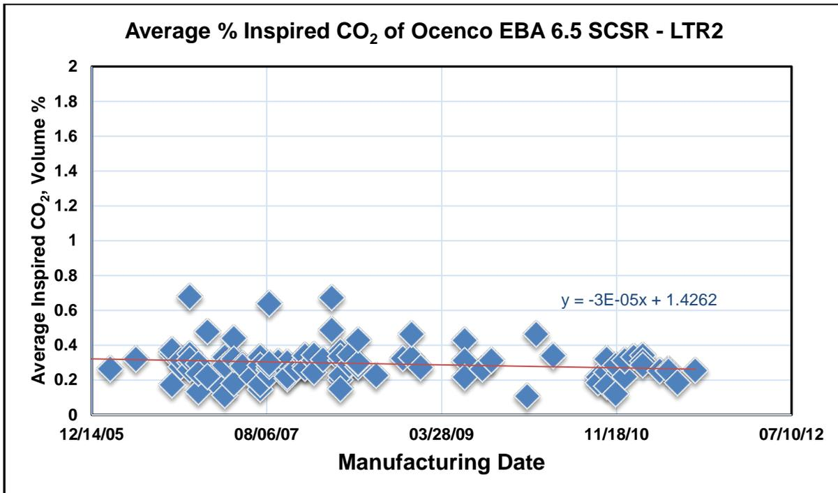
Figure 16. 60-Minute Average Percent Inspired Carbon Dioxide of Field Deployed and New Ocenco EBA 6.5 Self-Contained Self-Rescuers
