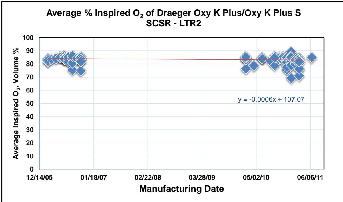
Figure 11. 60-Minute Average Percent Inspired Oxygen of Field Deployed and New Dräger Oxy K Plus/Oxy K Plus S Self-Contained Self-Rescuers
