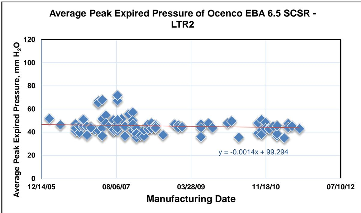
Figure 20. 60-Minute Average Peak Expired Pressure of Field Deployed and New Ocenco EBA 6.5 Self-Contained Self-Rescuers
