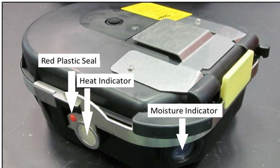
Figure 8. Areas of Visual Inspection for Dräger Oxy K Plus SCSR
