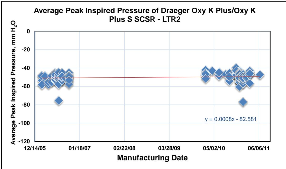
Figure 13. 60-Minute Average Peak Inspired Pressure of Field Deployed and New Dräger Oxy K Plus/Oxy K Plus S Self-Contained Self-Rescuers
