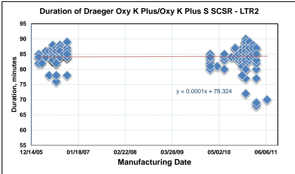
Figure 9. Duration of Field Deployed and New Dräger Oxy K Plus/Oxy K Plus S Self-Contained Self-Rescuers
