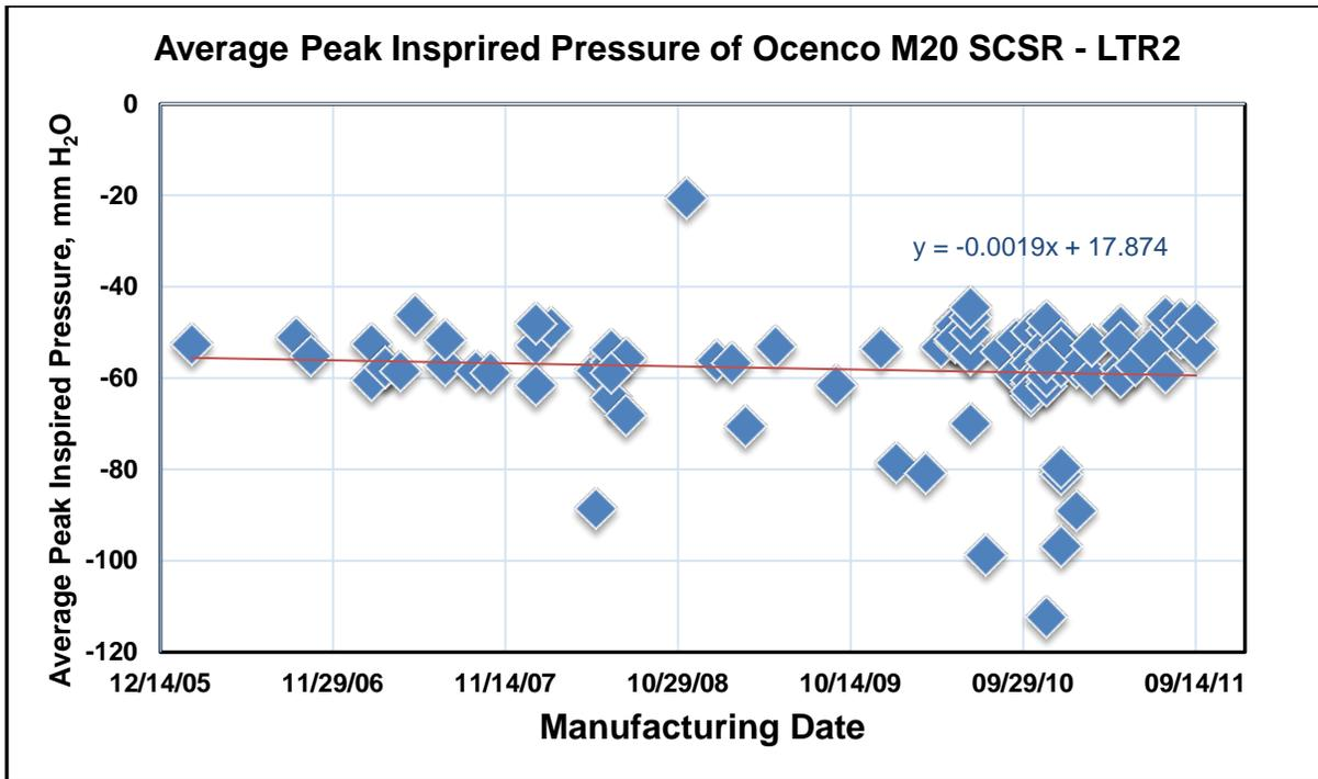
Figure 25. 10-Minute Average Peak Inspired Pressure of Field Deployed and New Ocenco M-20 Self-Contained Self-Rescuers
