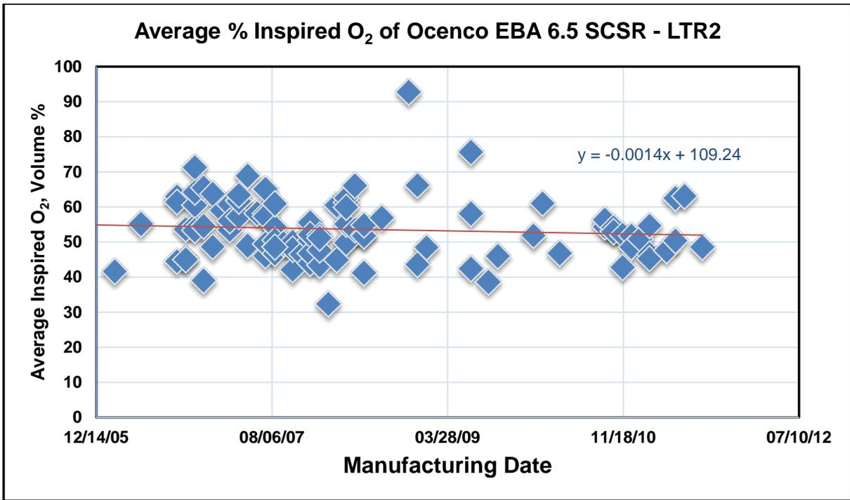
Figure 17. 60-Minute Average Percent Inspired Oxygen of Field Deployed and New Ocenco EBA 6.5 Self-Contained Self-Rescuers
