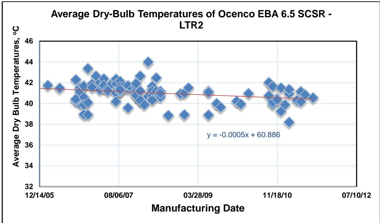
Figure 18. 60-Minute Average Dry-Bulb Temperatures of Field Deployed and New Ocenco EBA 6.5 Self-Contained Self-Rescuers
