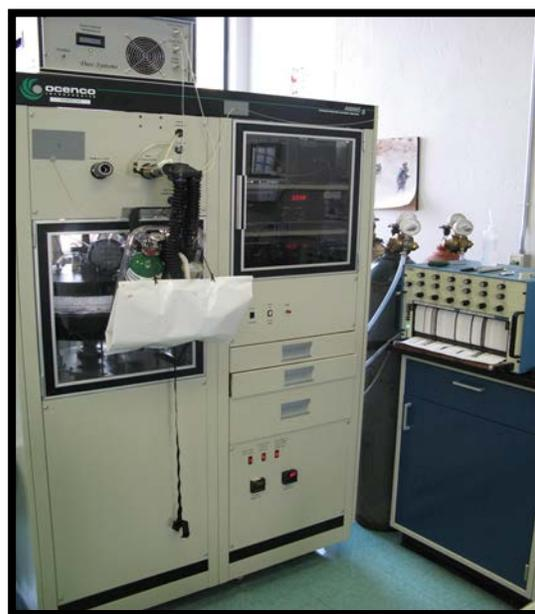
Figure 5. Automated Breathing and Metabolic Simulator
