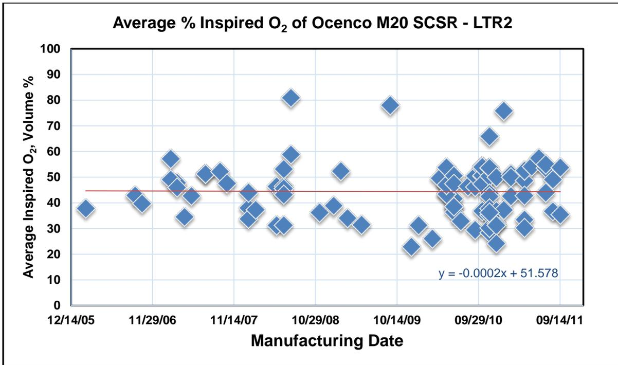
Figure 23. 10-Minute Average Percent Inspired Oxygen of Field Deployed and New Ocenco M-20 Self-Contained Self-Rescuers
