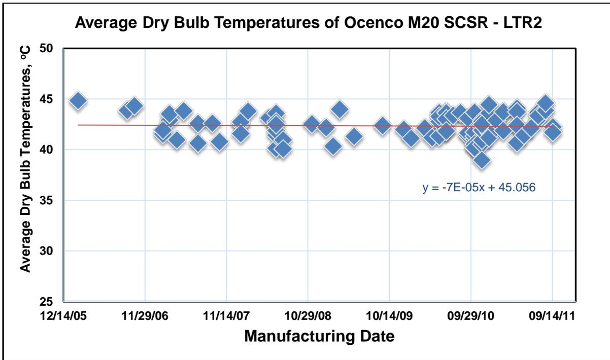
Figure 24. 10-Minute Average Dry-Bulb Temperatures of Field Deployed and New Ocenco M-20 Self-Contained Self-Rescuers
