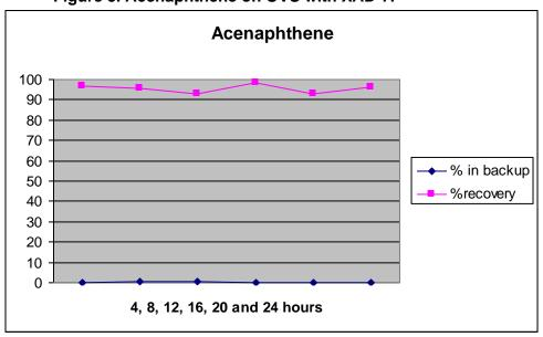
Figure 5. Acenaphthene on OVS with XAD-7.
