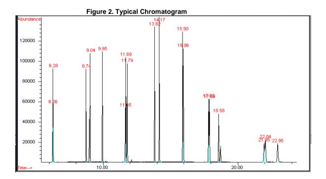
The mass spectrometer is operated in Selected-Ion Monitoring (SIM) mode using a dwell time of 30 ms for each ion. Six different SIM windows are used as shown in Table 4. Table 5 lists ions to use for quantitation, ions for spectral confirmation and internal standard references.
