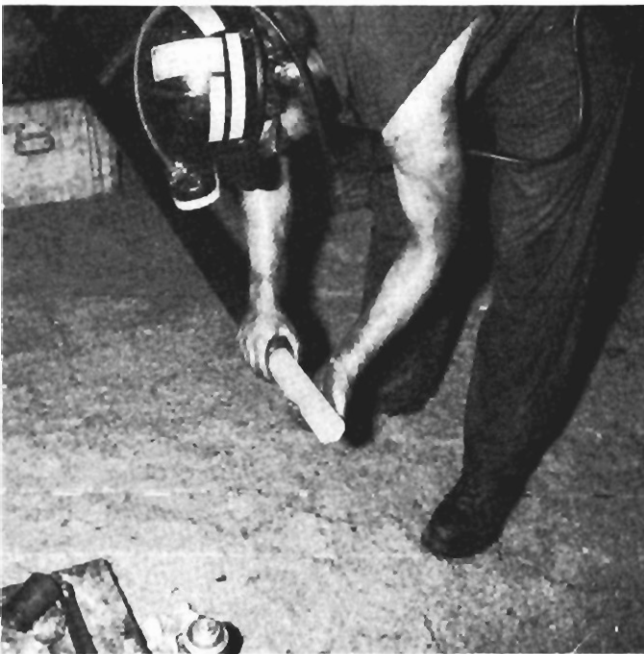
FIGURE 25. - Salt core recovered from exploratory drill holes. Cores were physically inspected and bagged for methane content test.
