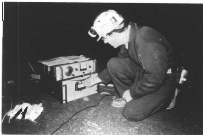
Fig. 1. Fire warning system transmitter.
