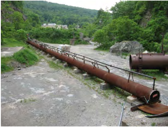
Figure 1—NIOSH LLL explosion tube with control building in the distance.
