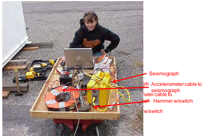
Figure 2. Photograph at the Spokane Research Laboratory concrete block test site showing the arrangement of the recording system on a coaster wagon.
