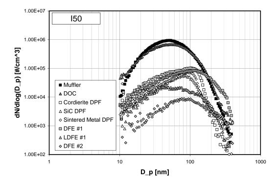
Figure 6. Aerosol size distribution measured during I50 tests
