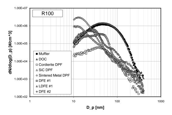
Figure 5. Aerosol size distribution measured during R100 tests
