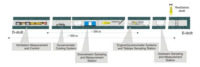
Figure 2. NIOSH Diesel Laboratory in D-drift of LLL
