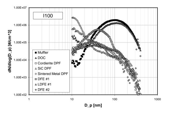
Figure 7. Aerosol size distribution measured during I100 tests
