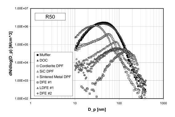
Figure 4. Aerosol size distribution measured during R50 tests
