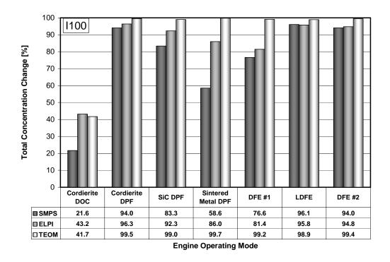
Figure 11. Percentage of total number and mass concentrations change for I100 test modes The results indicate the following:
