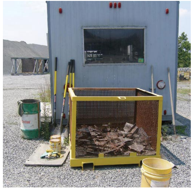
Basket for storing metal scrap that can be moved with a forklift.
