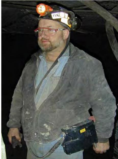
**Figure 39.** Miner wearing personal dust monitor (PDM).
