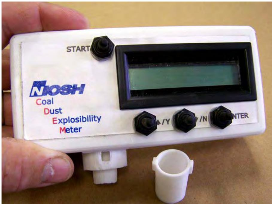
**Figure 41.** Coal Dust Explosibility Meter.
