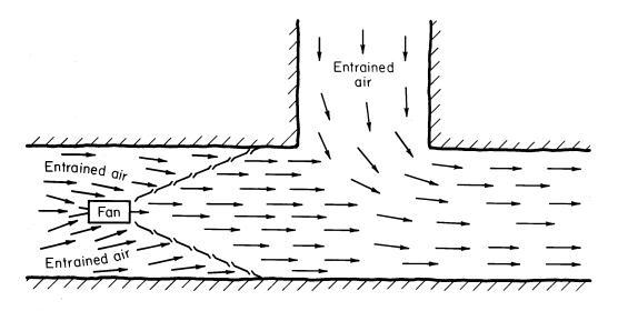
Figure 4-3.—Jet fan entrainment of mine air.
