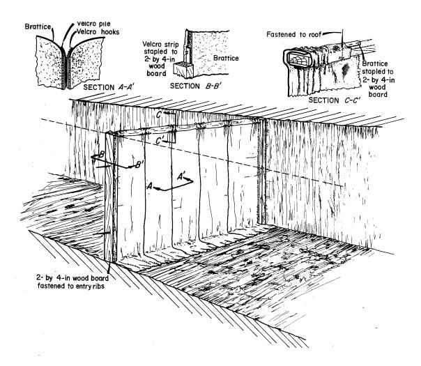
Figure 4-6.—Stopping built from damage-resistant brattice.
