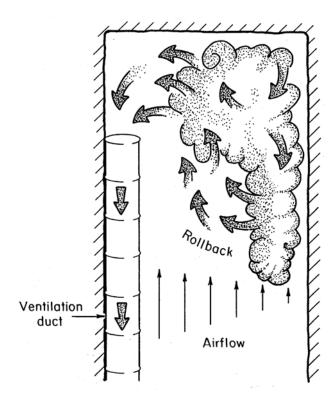
Figure 1-1.—Rollback of dust resulting from non-uniform airflow.
