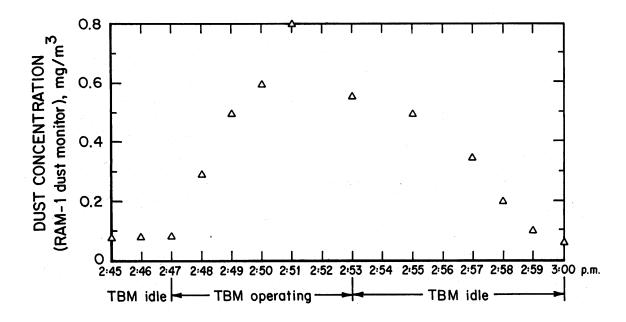
Figure 7-2.—Dust concentration measured near cutter head with TBM idle and operating.
