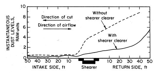
Figure 3-3.—Typical respirable dust concentration profile around the shearer during the tail-to-head pass.
