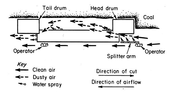
Figure 3-4.—Air currents when using the shearer-clearer system.
