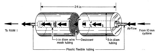
Figure 8-1.—Mist eliminator for direct-reading instruments that use light scattering [Cecala et al. 1985].
