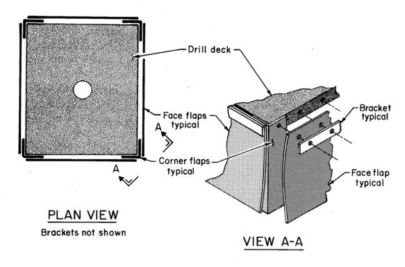
Figure 5-1.—Corner flaps added to a deck shroud to reduce leakage.
