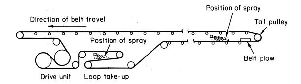
Figure 6-3.—Wetting both surfaces of the bottom belt.
