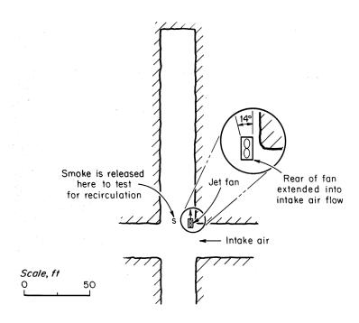
Figure 4-2.—Jet fan ventilating a single straight heading.
