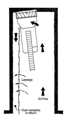
Figure 8-3.—Air in return diluted by line curtain leakage [Kissell et al. 1986].
