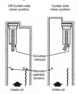
Figure 2-4.—Dust scrubber used with exhaust ventilation.
