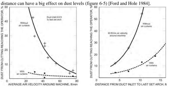
Figure 6-5.—Effect of duct inlet position, air velocity, and air curtain use on dust levels (from Ford and Hole [1984]).
