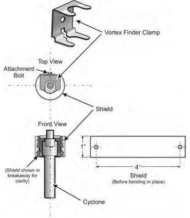
Figure 8-4.—Cyclone shield for high-velocity air streams.
