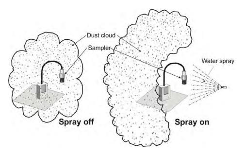
Figure 1-5.—Water spray test that can lead to overrating spray effectiveness.
