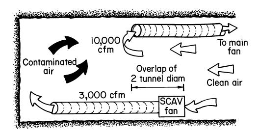
Figure 7-3.—Auxiliary, or scavenger, system with adequate overlap.
