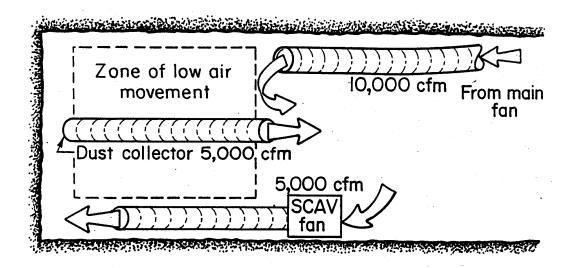
Figure 7-6.—Zone of low air movement is created because ducts have similar air quantities moving in opposite directions.
