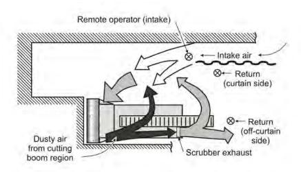
Figure 2-3.—Excessive air blown toward the face will cause dust to bypass the scrubber inlets.
