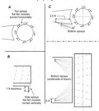
Figure 2-7.—Antirollback water spray system.
