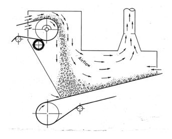
Figure 6-4.—Dust-laden air exhausted from transfer point enclosure.
