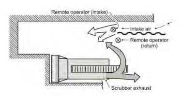
Figure 2-2.—Dust scrubber used with blowing ventilation.
