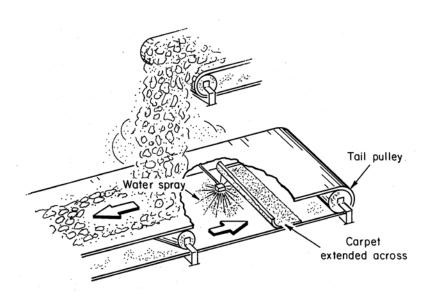
Figure 6-2.—Wetting the top surface of the bottom belt.
