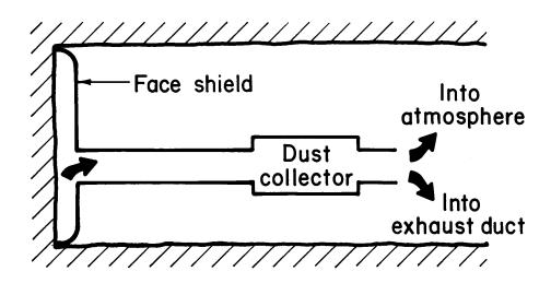
Figure 7-7.—TBM dust collection system.
