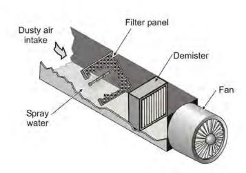
Figure 2-1.—Machine-mounted scrubber design.
