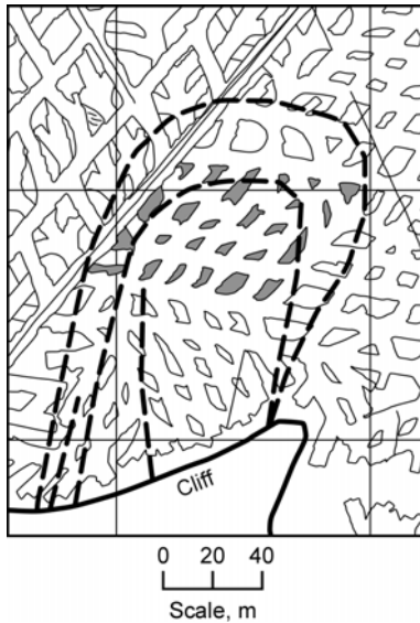
Figure 2. Collapsed pillars (shaded) and surface cracking (dashed lines) at a Phosphate mine (13).
