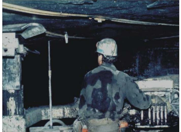
Figure 3.—Installing a roof bolt in an underground coal mine.
