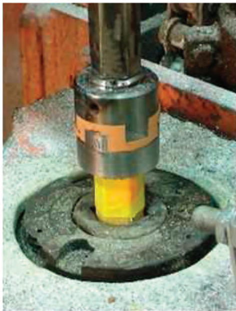
Figure 3 — Jaw-type coupling with 58 Shore D urethane spider.
