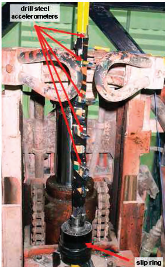
Figure 1 — Drill steel accelerometers and slip ring assembly.
