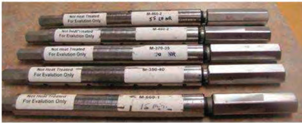
Figure 8 — Isolators bonded with elastomers from Table 5.
