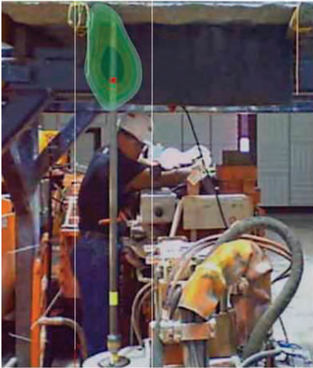
Figure 5 — Beamforming results for drilling with the jaw-type coupling, 96 dB(A) at the operators' position.
