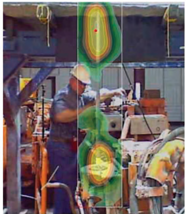
Figure 4 — Beamforming results for baseline drilling, 100 dB(A) at the operator's position.
