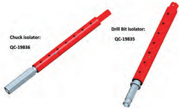
Figure 6 — Final production designs of isolators for use with 35-mm-diameter drill bits.
