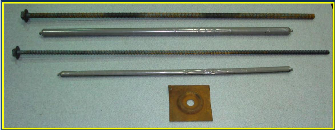
*Fig. 2 - Resin and roof bolts, 3.5 cm (1.375-in) [top], 2.5 cm (1-in) [middle] and plate [bottom].*
