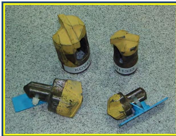
*Fig. 4 - Drill bits, vacuum [top] and wet or mist [bottom].*
