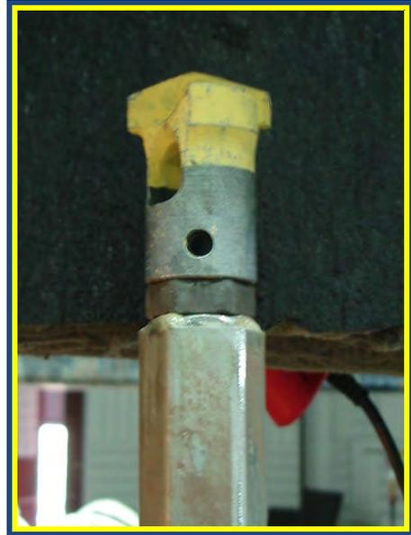
*Fig. 9 - Damped hexagonal drill steel and 4.1 cm [1.625-in] bit*
