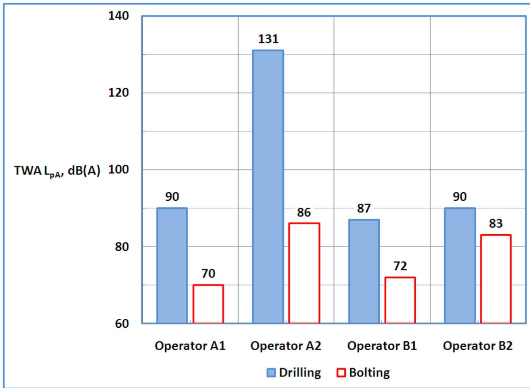
*Fig. 5 - RBM operators noise levels during drilling and bolting.*
