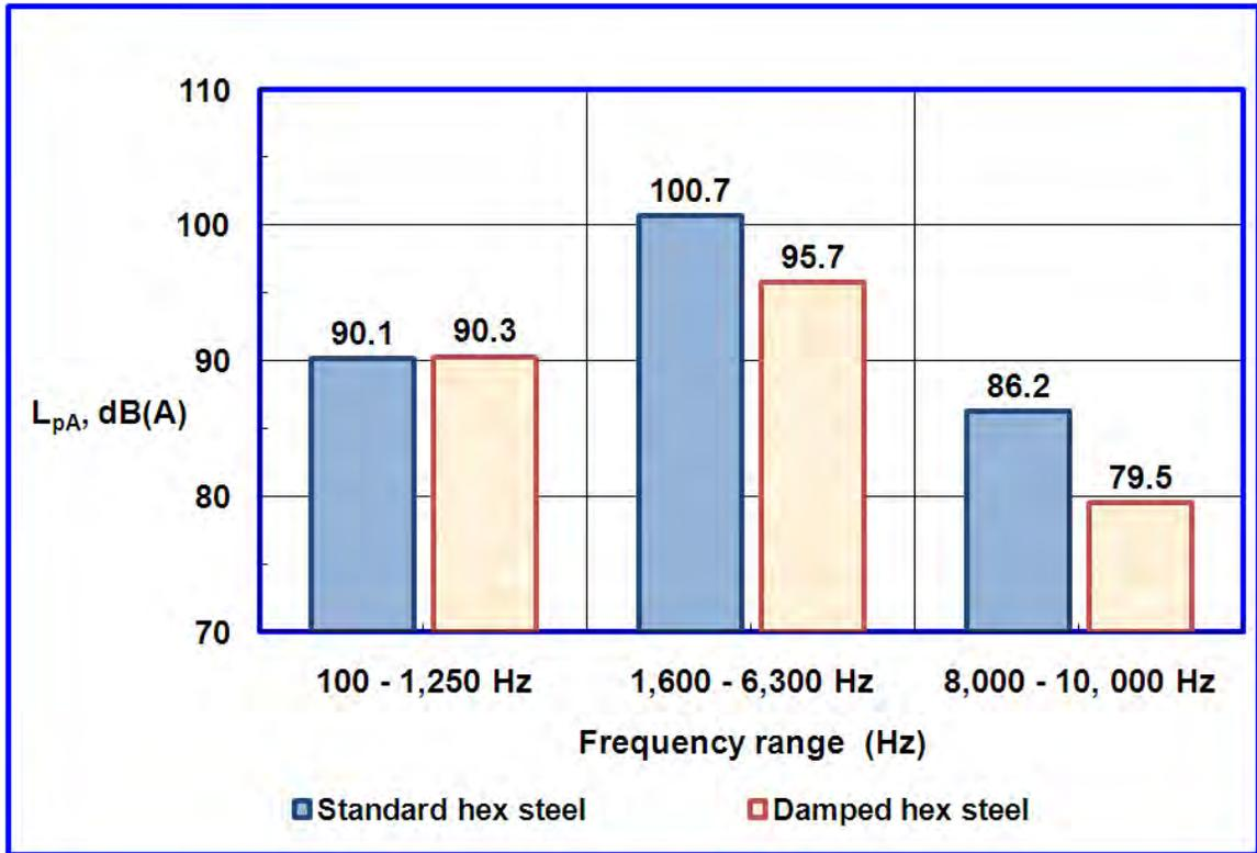
Fig. 14 – A-weighted sound power level contributions of selected frequency ranges.
