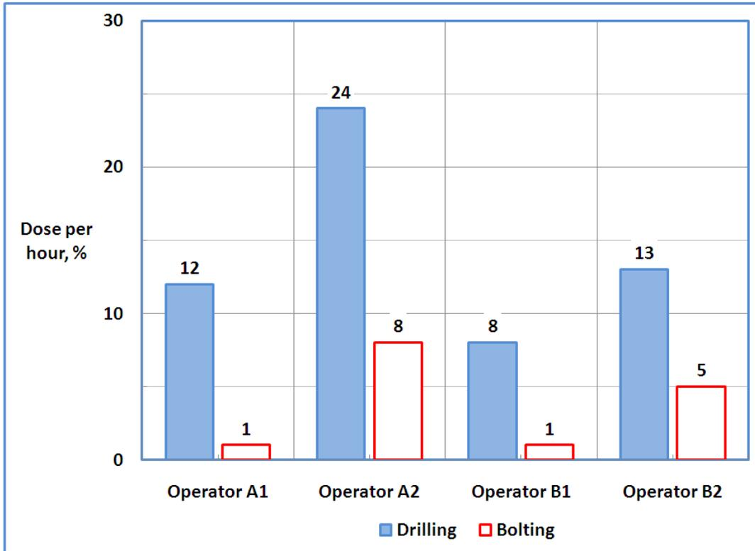
Fig. 6 - RBM operators dose accumulation rate when drilling and bolting.
