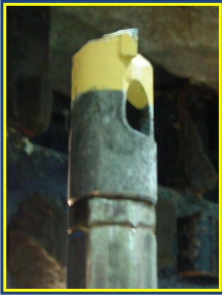
*Fig. 8 - Standard hexagonal drill steel and 4.1 cm [1.625-in] bit*
