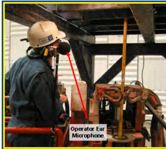
*Fig. 10 - Operator ear microphone location.*
