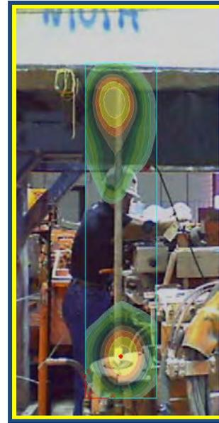
Fig. 12 - Beamforming data collected during damped hexagonal drill steel testing.
