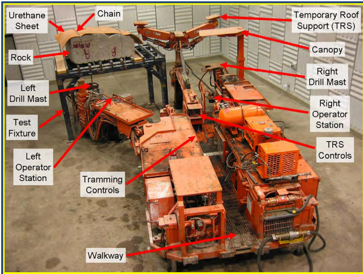
*Fig. 1 - Roof bolting machine and drill media located in the hemi-anechoic chamber.*
