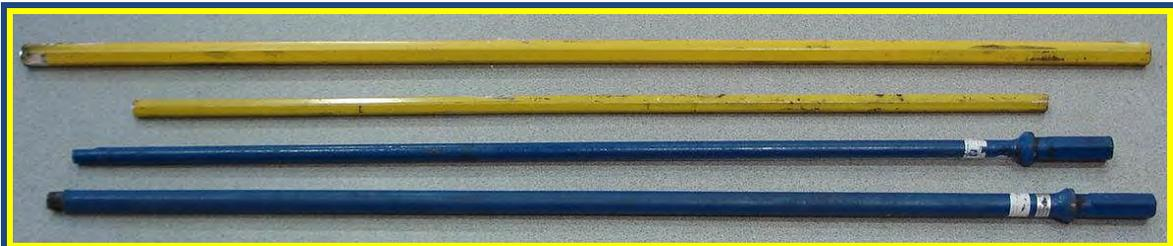
*Fig. 3 - Drill steels, hexagonal [top], and round [bottom].*
