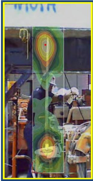
Fig. 11 - Beamforming data collected during standard hexagonal drill steel testing.
