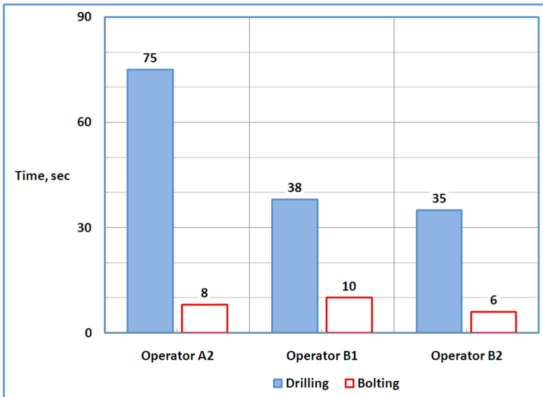
Fig. 7 - RBM operators average time to drill and bolt a hole.
