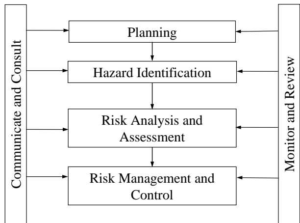
Figure 2. Risk management process to mitigate roof fall injury (after MOSHAB, 1999).
