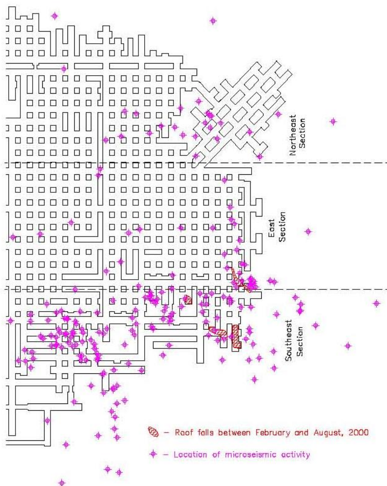
Locations of 1,302 microseismic events recorded from Feb. 9 through Aug. 31, 2000, and contained within the northeast, east and southeast sections.
