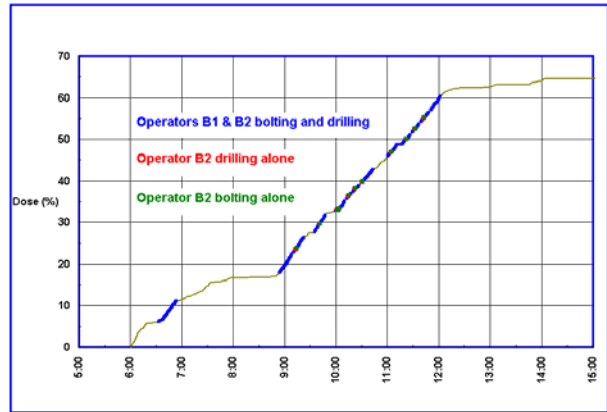
Figure 7: Noise dose accumulation, operator B2, portal B
