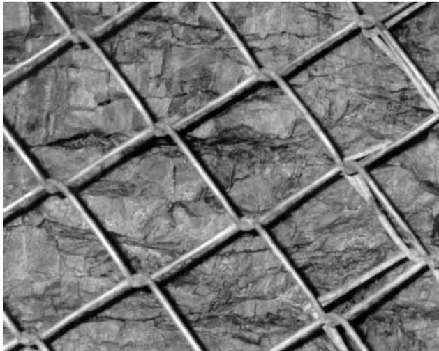
Figure 5. Mining-induced extension fractures in stope walls.
